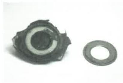
Nut with Top side of Broken T-bolt still inside
