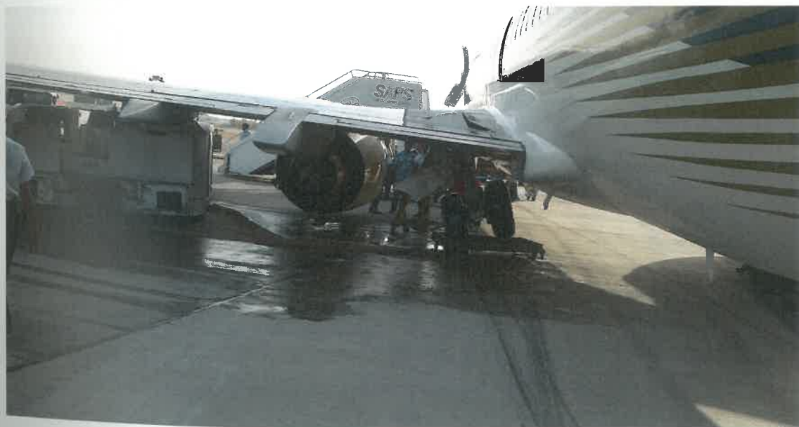
Collapsed LHS Main Landing and Engine No 1 resting on runway surface
