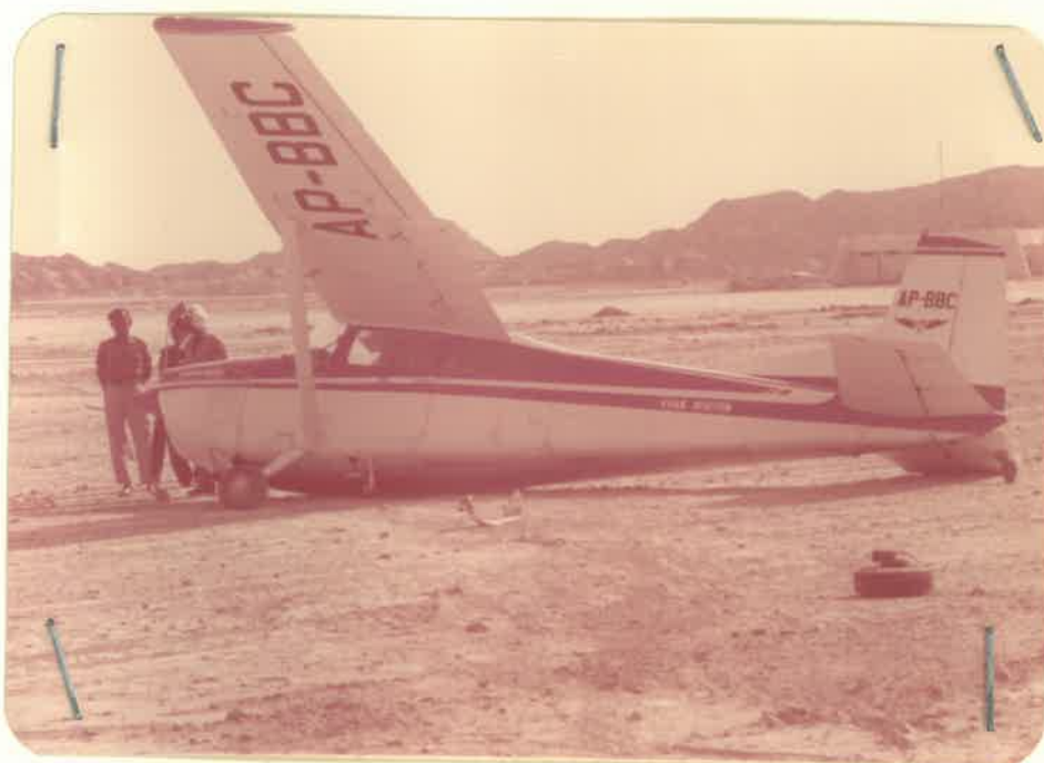
A view of the wreckage from left hand side. Please note port wheel and tail wheel are in tact. In the fore ground the damaged starboard tyre and wheel broken-off can be seen. The starboard landing gear spring and axle can be seen just below the aircraft fuselage.
