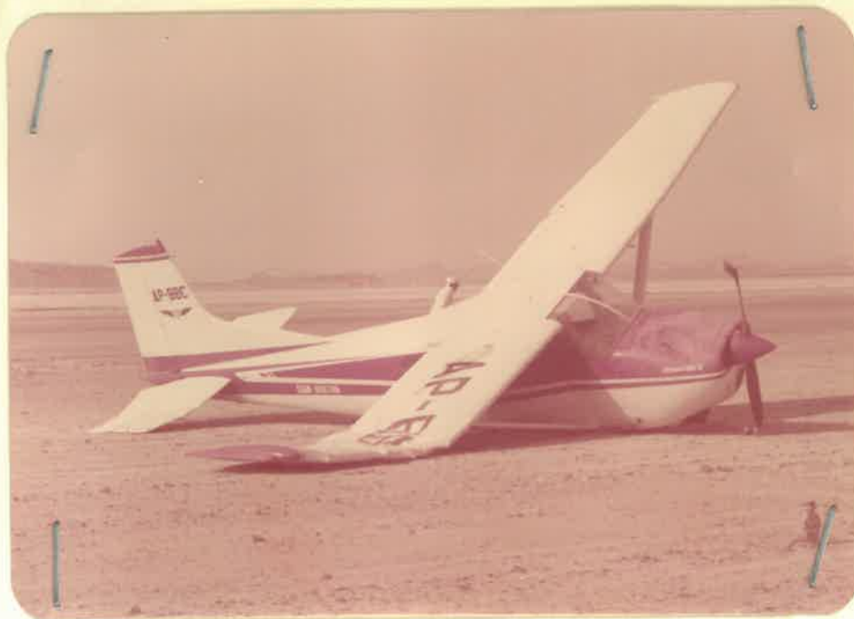
A view of the wreckage of Cessna 185F. Nationality and Registration Mark AP-BBC can be seen clearly. Please also note propeller. The tip of the upper blades has broken-off.
