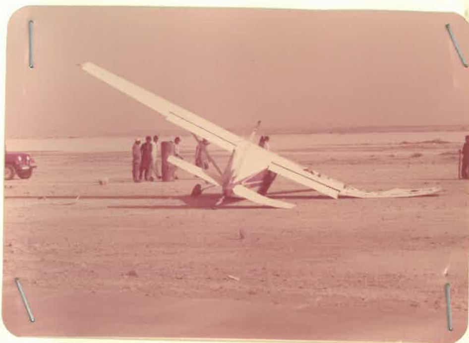
4 Rear view of the wreckage. Please note tail wheel and damage to starboard tail plane and elevator. Also note position of flaps which are set for take-off.
