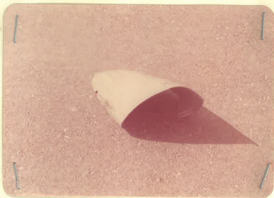
9 The tip of the propeller blade which had separated after the impact with the soft ground after the aircraft left the runway. No marks of propeller were evident on the runway surface.
