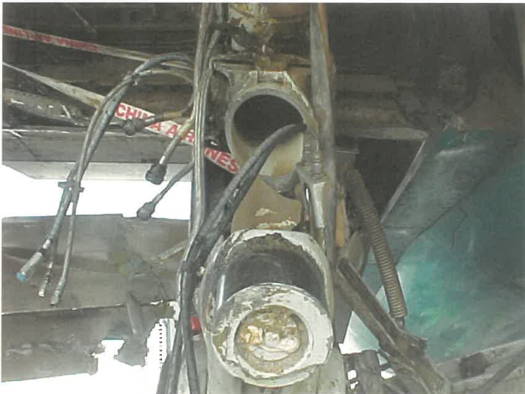
HINGE ARM FAILURE (SEPARATED FROM AIRCRAFT)
