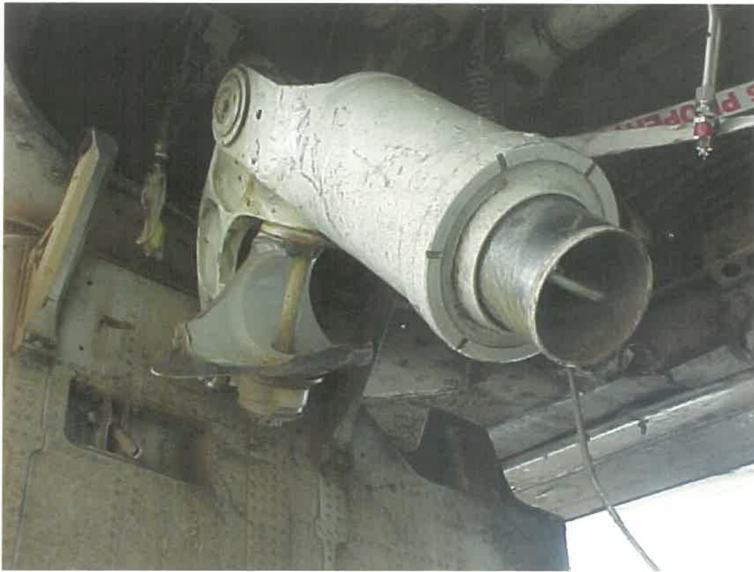
HINGE ARM FAILURE (ATTACHED TO AIRCRAFT)
