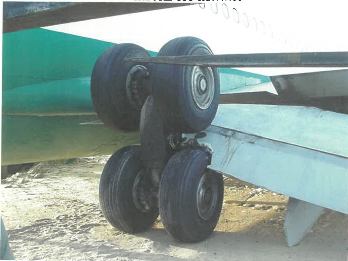
LANDING GEAR AFTER COLLAPSE
