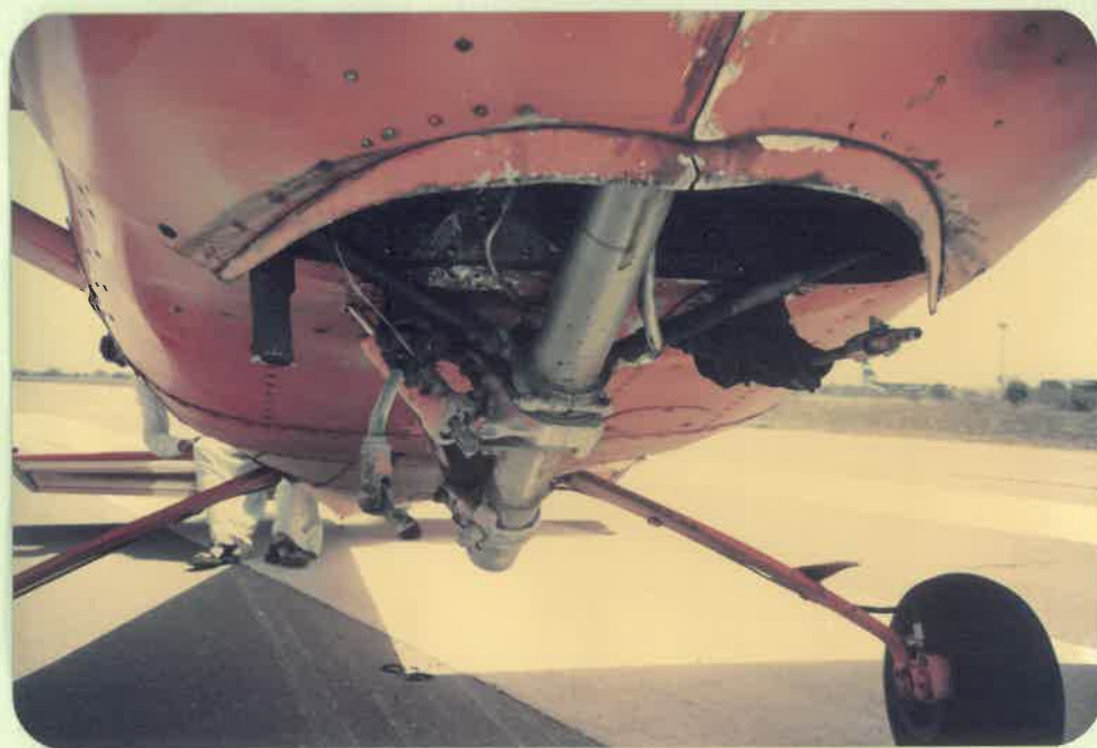
Photograph showing damage to the nose wheel strut and the point where the nose wheel broke.
