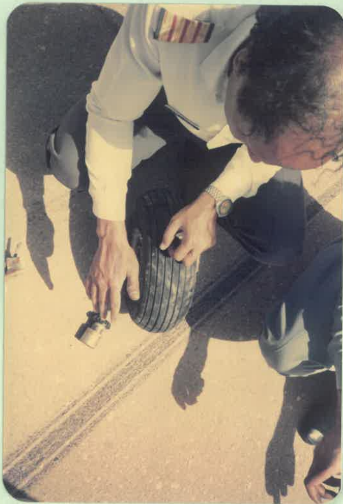
Deflated nose wheel with its components.
