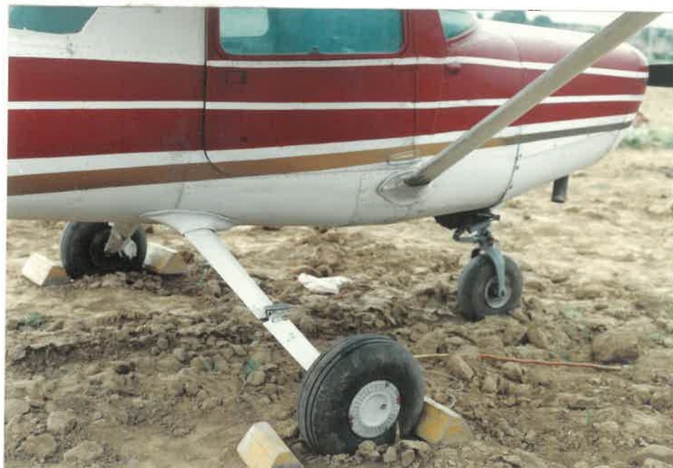
CLOSE-UP VIEW: NO DAMAGE CAUSED TO THE LANDING GEARS
