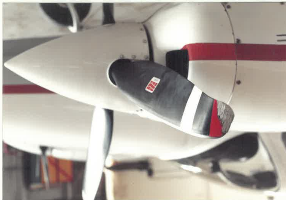
RIGHT ENGINE PROPELLER BLADE DAMAGE ANOTHER VIEW
