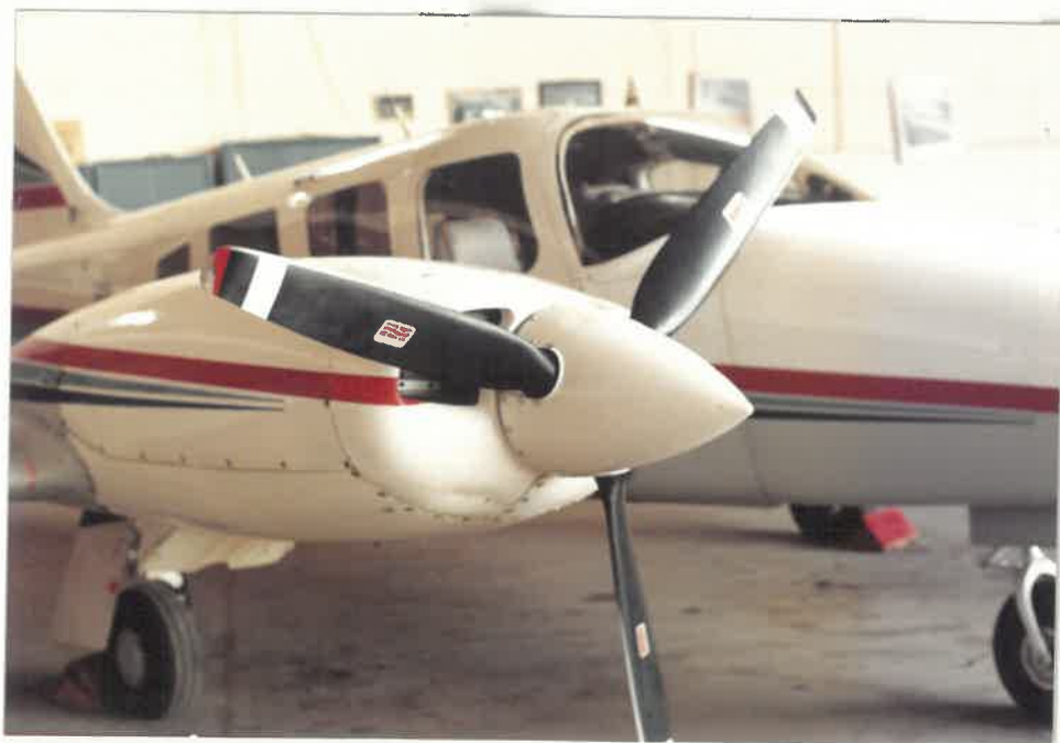
RIGHT ENGINE PROPELLER BLADES DAMAGED
