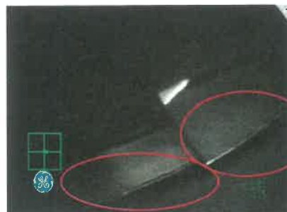
1 st Stage H.P.C. Blades with clappers With tip rubbed
