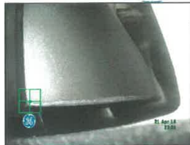
9 th Stage H.P.C. Blade with uneven clearance and tip rubbing
