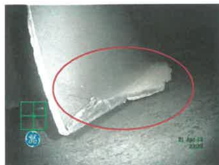
2 nd Stage H.P.C. Blade with rubbing from tip and tip curled as well
