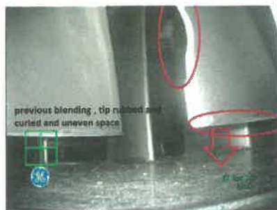
6 th Stage H.P.C. Blade with uneven clearance and tip erosion
