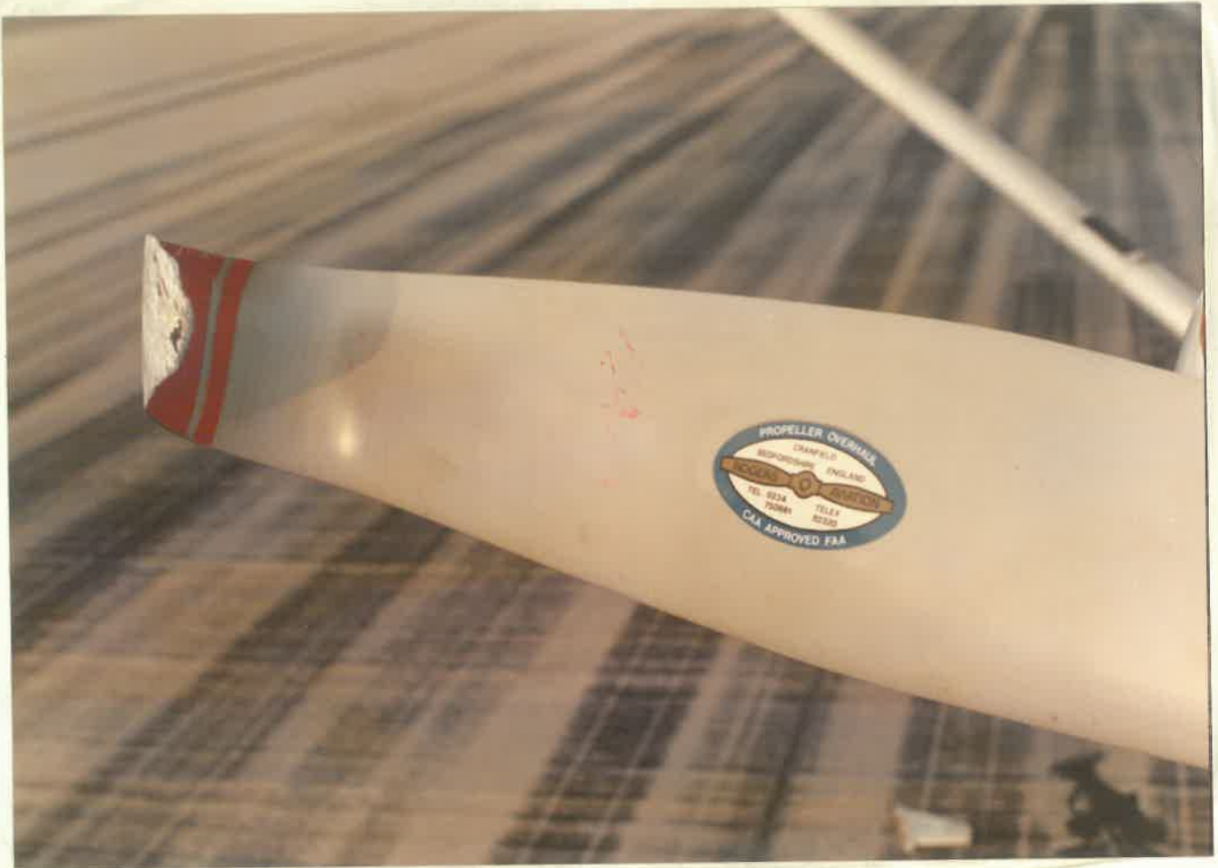
3. Damaged Prop TIP
