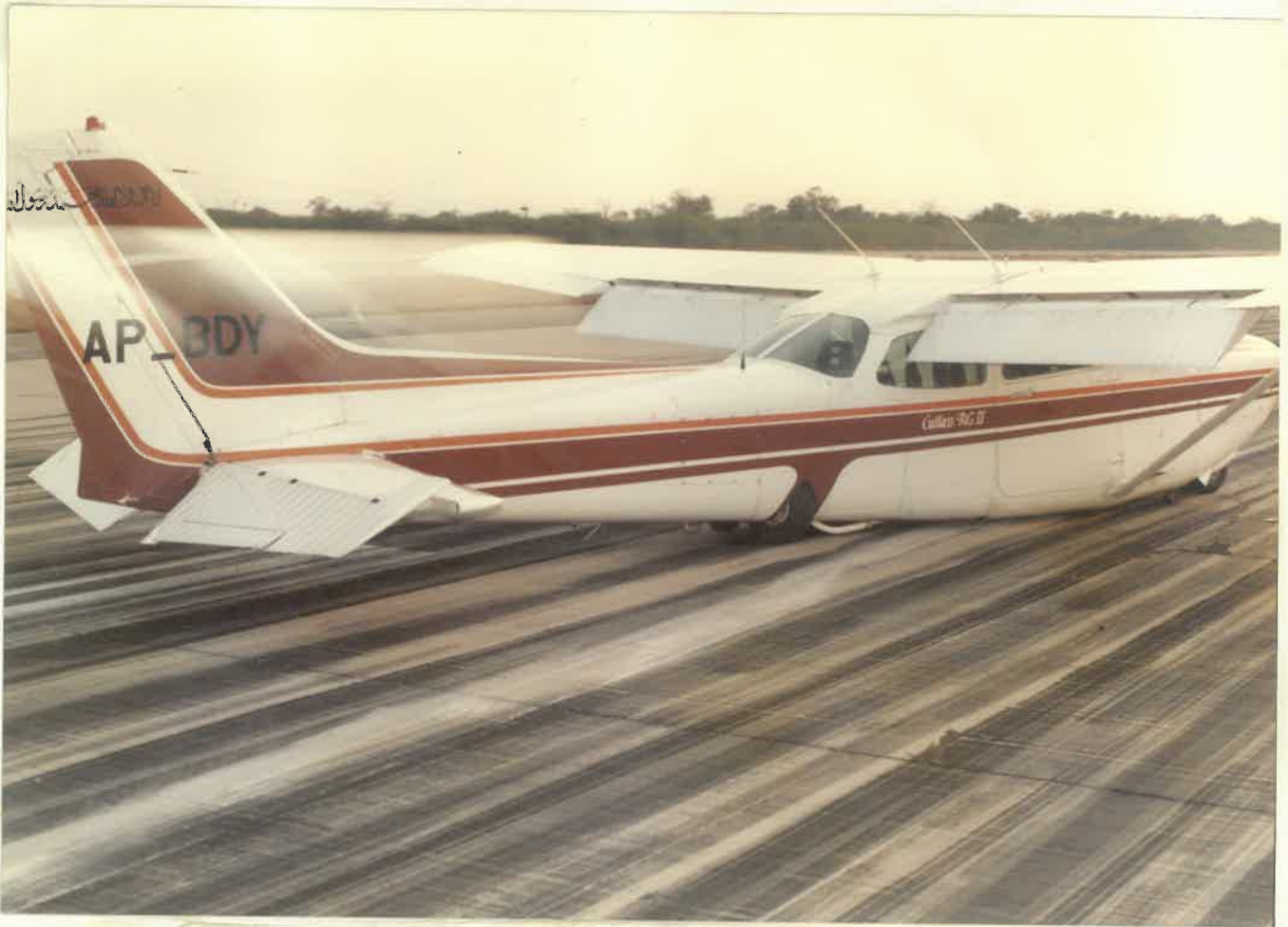
5. Main Wheels and Nose Gear in the process of coming "DOWN" - Flaps selected down about 30°.
