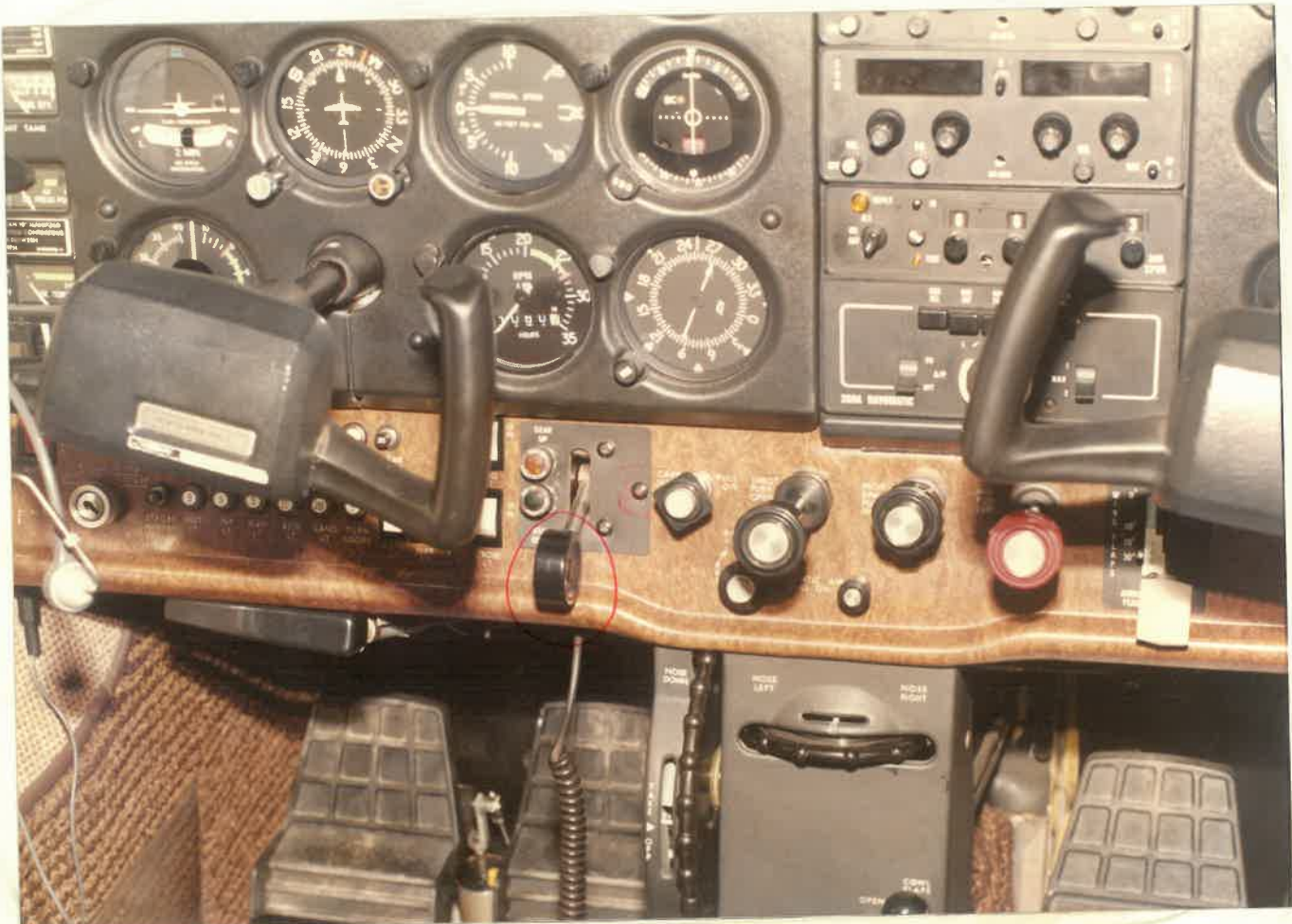
4. Cockpit Panel - indicating Gear-Lever Position "DOWN"
