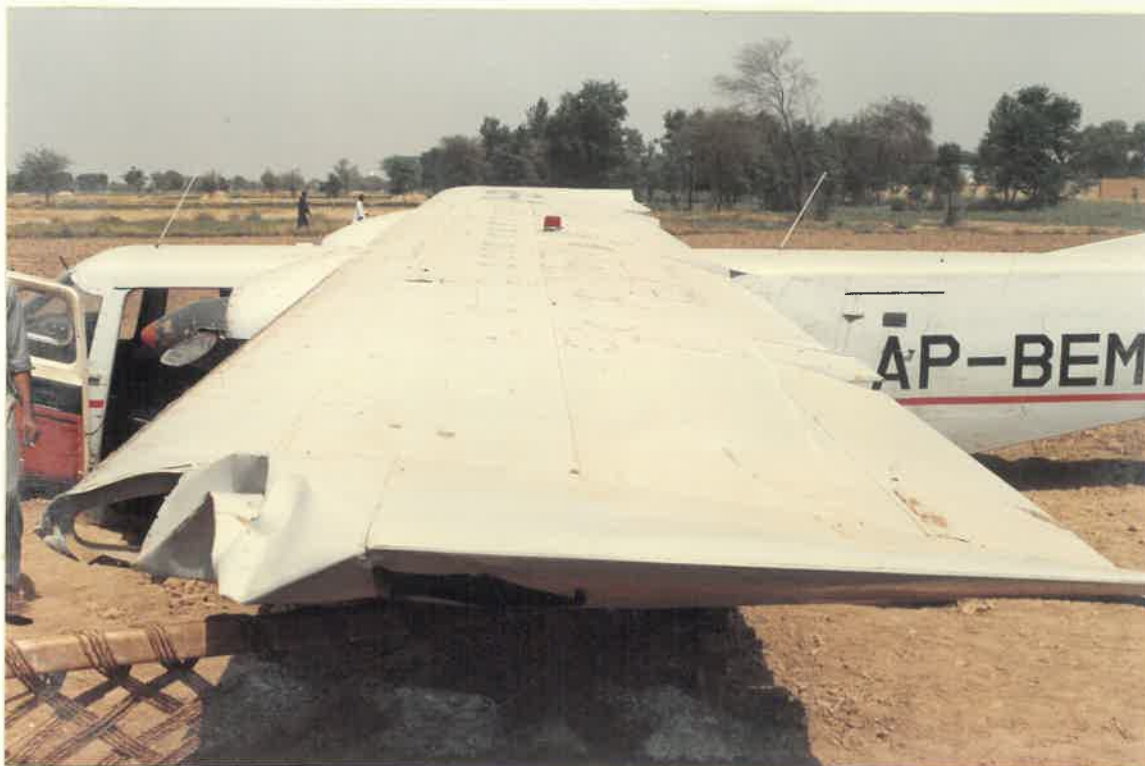
LEFT WING TIP DAMAGED (SIDE VIEW)
