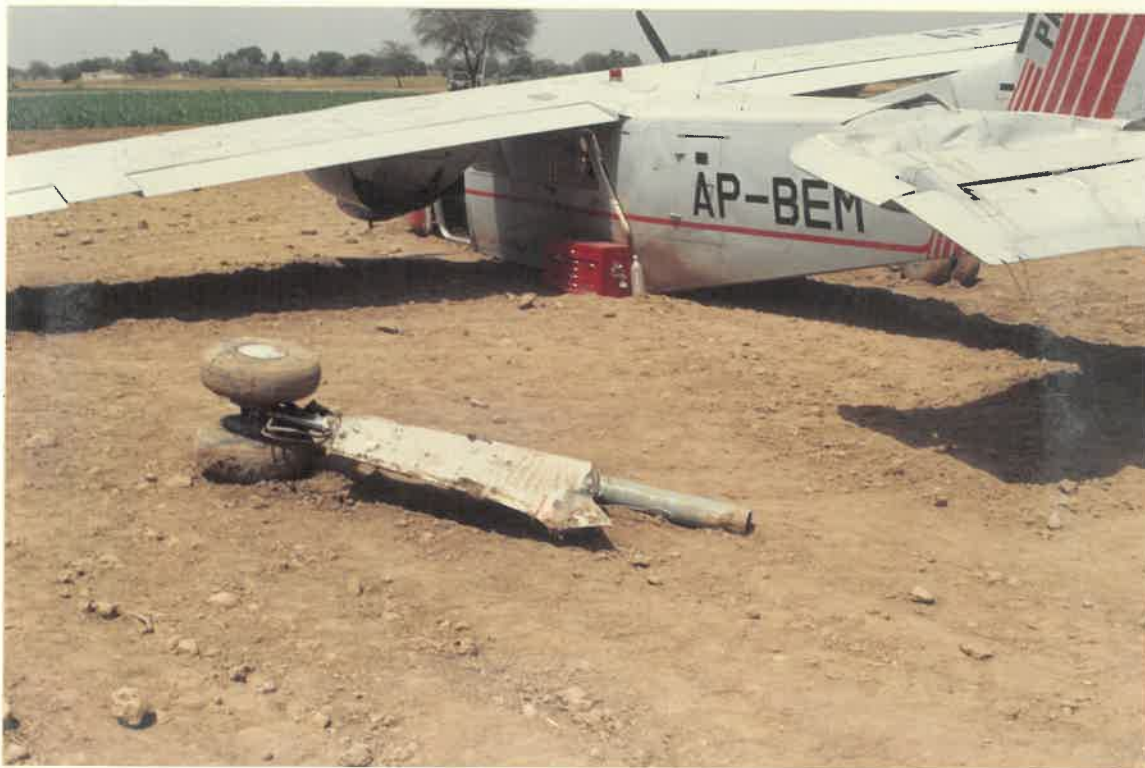
LEFT UNDER CARIAGE BROKE FROM ITS MOUNTING BASE
