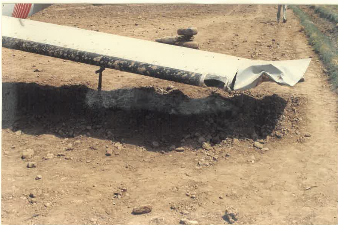
LEFT WING TIP DAMAGED (FRONT VIEW)
