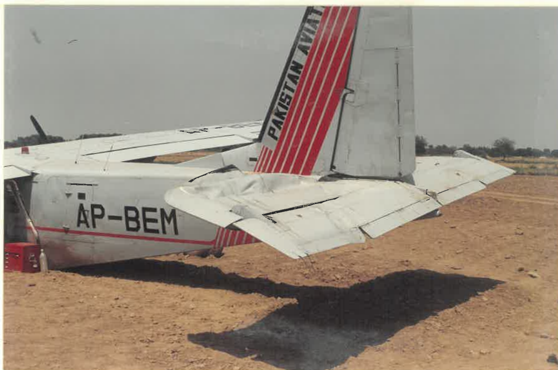
LEFT HORIZONTAL STABILIZER AND FLEVATOR DAMAGED
