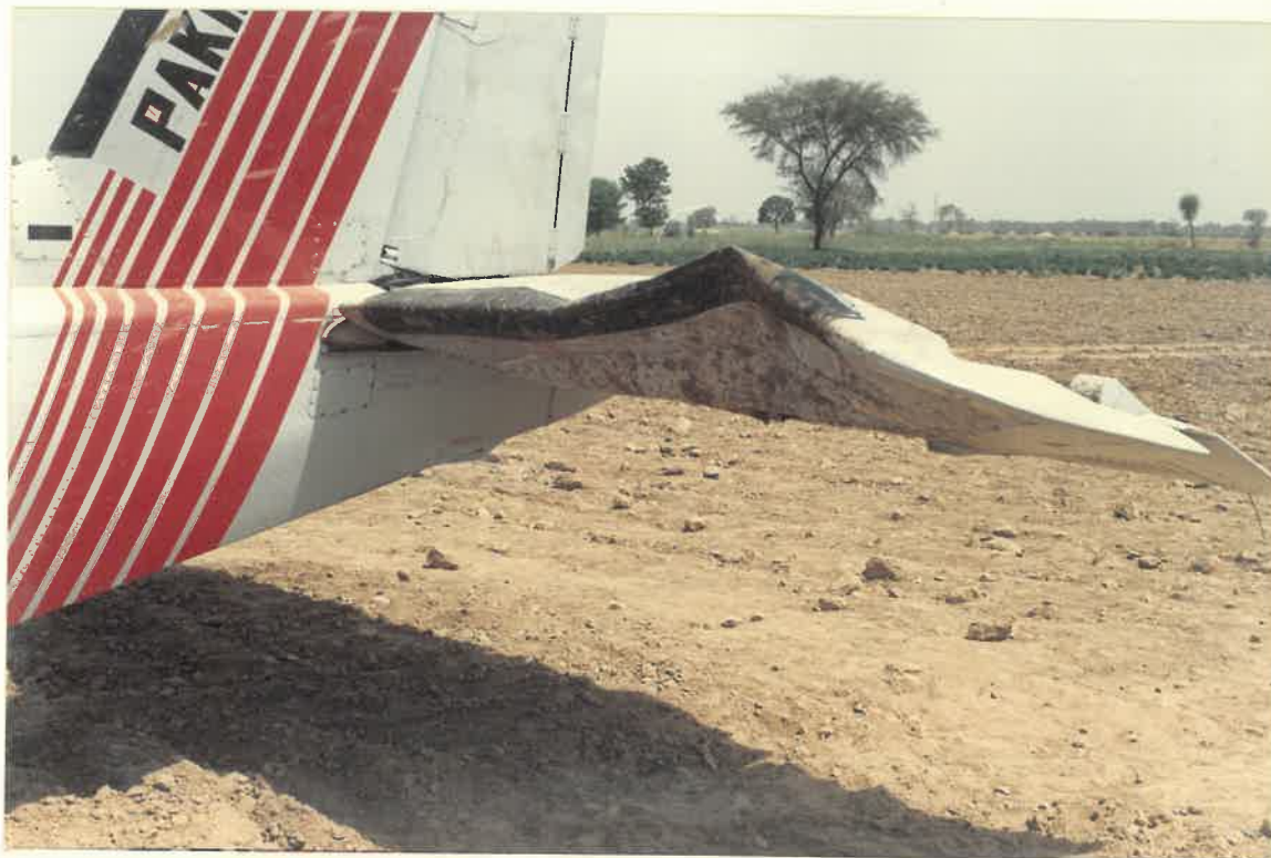
LEFT HORIZONTAL STABILIZER DAMAGED
