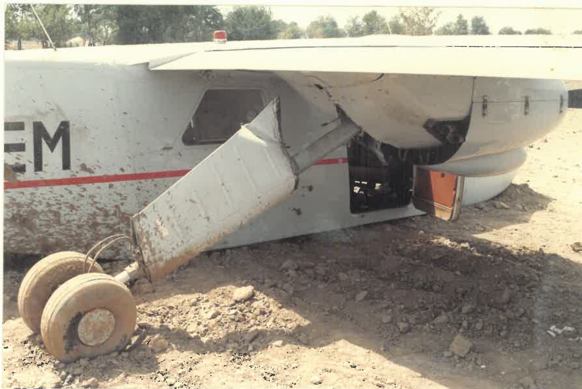
RIGHT UNDER CARIAGE BROKE FROM ITS MOUNTING BASE
