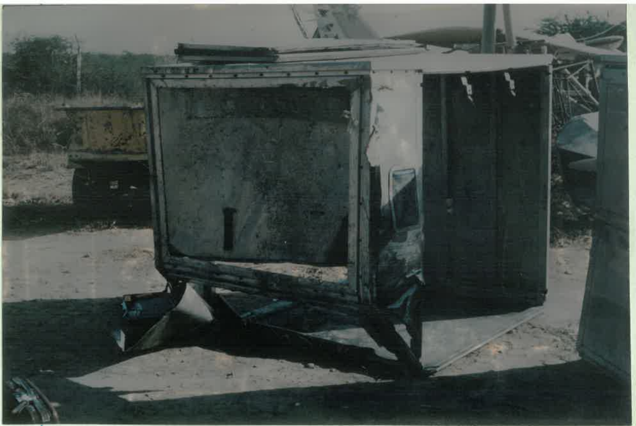
6. Photograph of the damaged container No. AVE 1650AF in which the explosion occurred.
