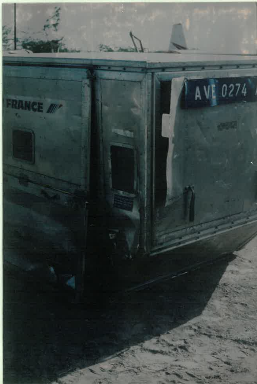
7. Photograph of the container No. AVE 0274 AF which was placed next to container AVE 1650 AF and which was also damaged due to the explosion.
