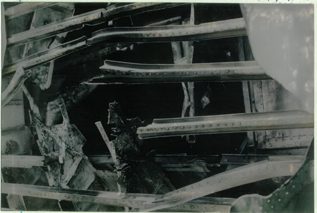
4. Photographs showing the factured ribs of the aircraft.
