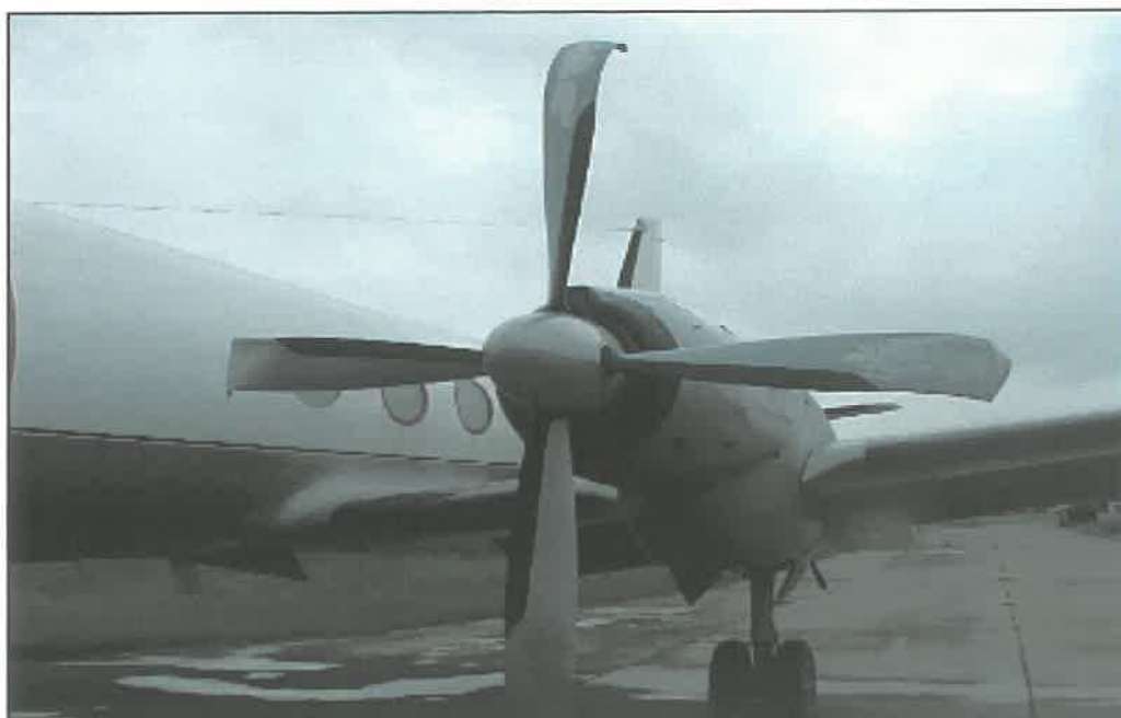
APPENDIX K8 PROPELLER TIP DAMAGE – A CONSEQUENCE OF HIGH RPM DURING LANDING
