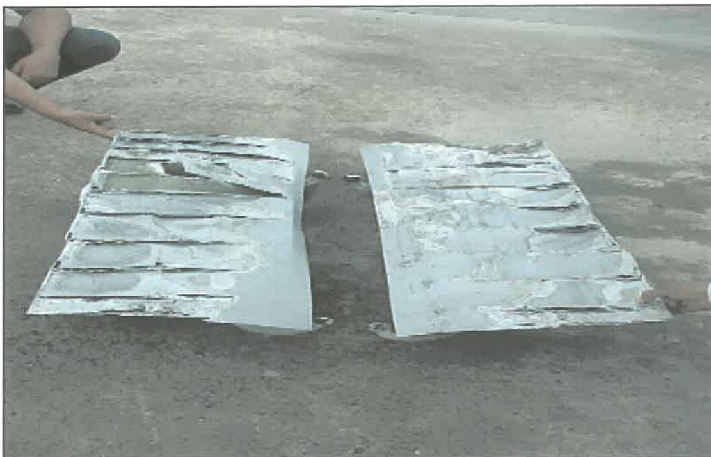
APPENDIX K6 LANDING GEAR DOORS – EXTERNAL DAMAGE – DUE TO CONTINUOUS GROUND RUBBING
