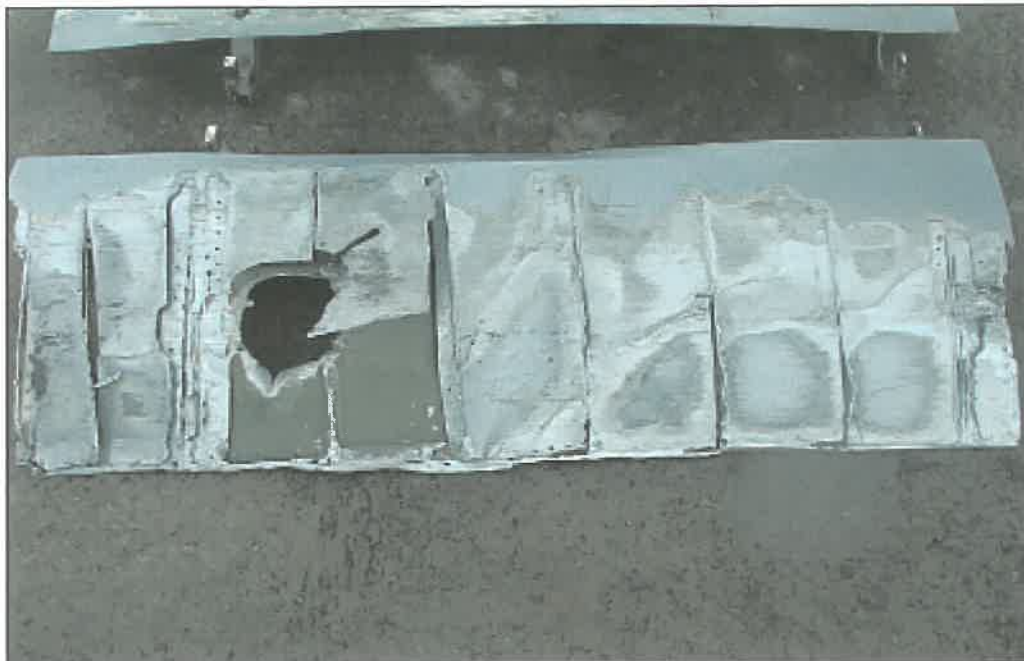
APPENDIX K7 LEFT NOSE LANDING GEAR DOWN – EXTENT OF DAMAGE DUE TO GROUND RUBBING
