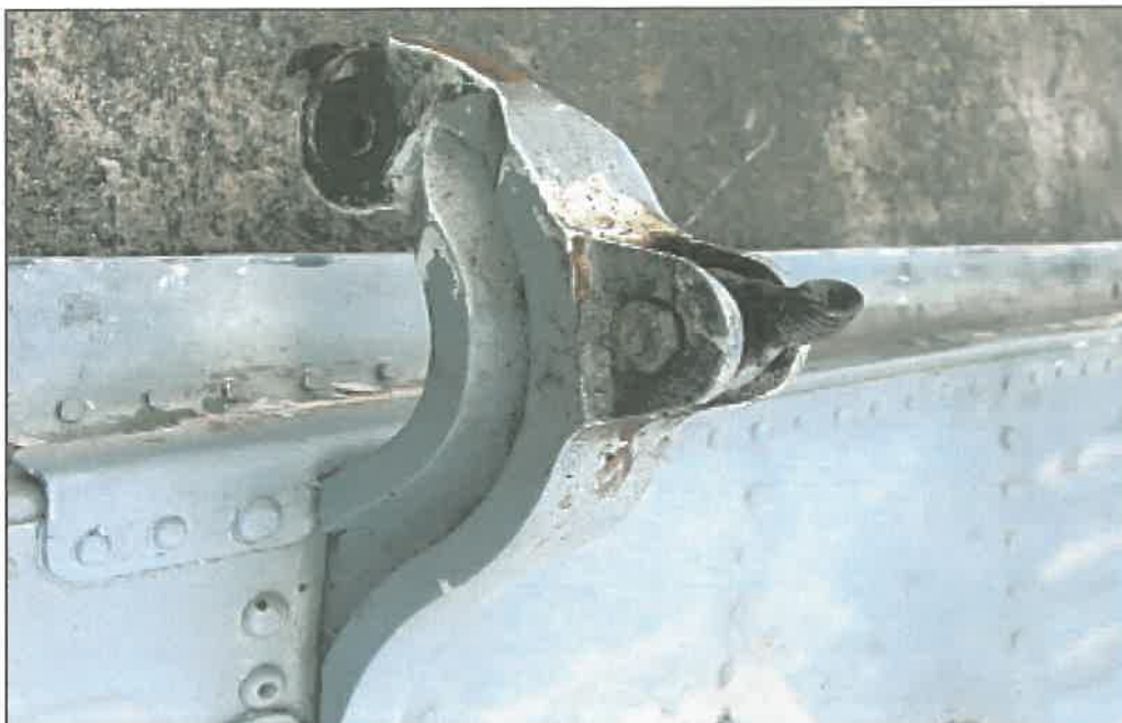
APPENDIX K5 RIGHT NOSE LANDING GEAR LINK ROD BROKEN END SHOWING BENDING AT THREADED END BEFORE FAILURE DURING IMPACT
