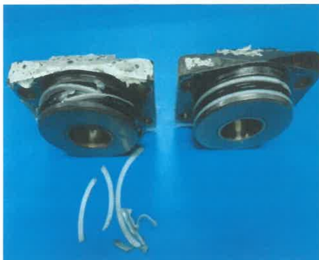
Damaged vs Intact Ring Backup
