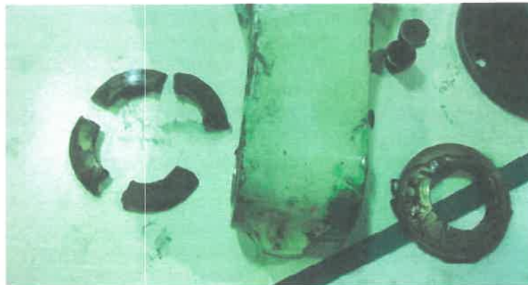
Lower Torsion Link upper lug damaged and intact bush
