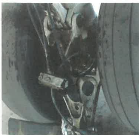
Fractured Upper Torsion Link and damaged Shimmy Damper
