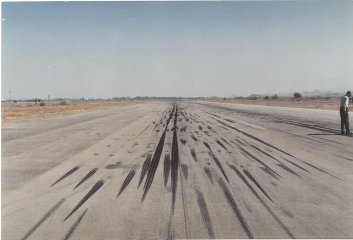
LEFT TYRE MARKS UPTO POINT OF BURST
