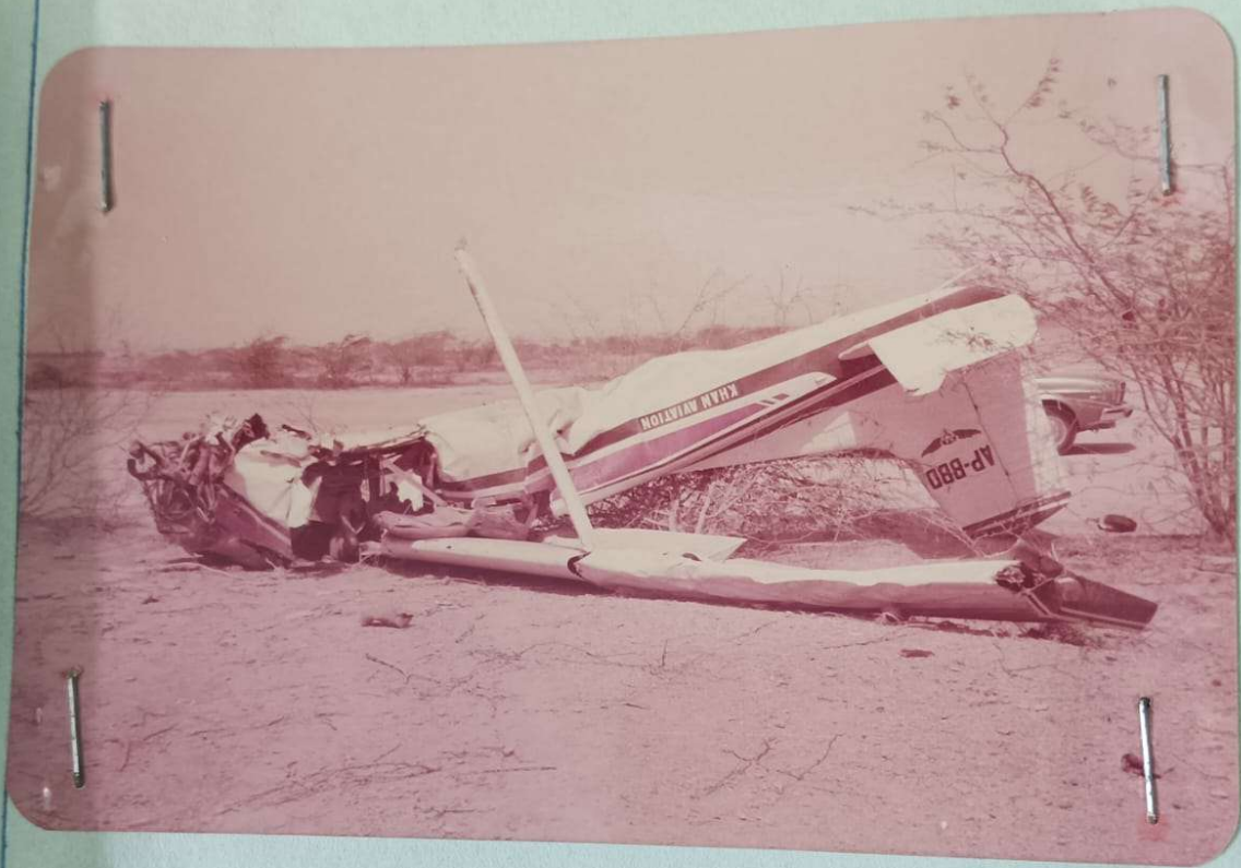
THE VIEW OF THE MAIN WRECKAGE WHERE IT CAME TO REST NOTE THE DAMAGE TO THE COCKPIT AND THE RIGHT TAIL F THE REGISTRATION MARK CAN CLEARLY BE SEEN. NOTE THE POSITION OF THE FLAP.
