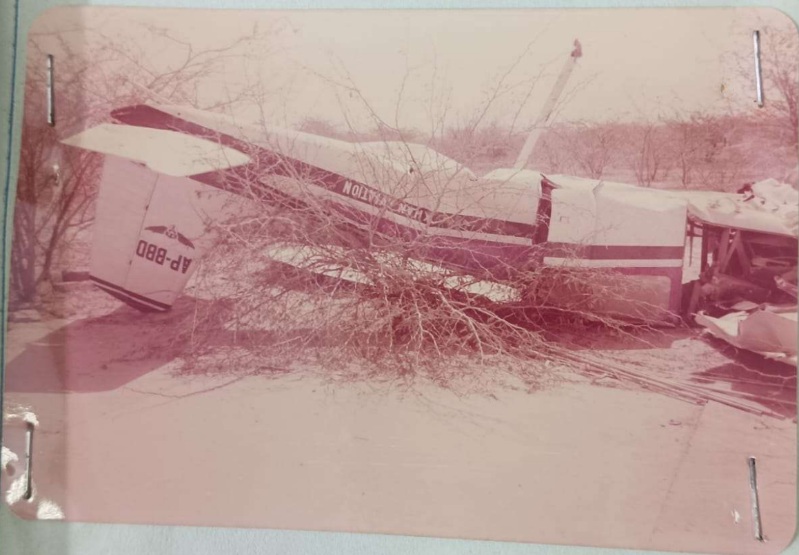
A VIEW OF THE WRECKAGE FROM THE LEFT HAND SIDE. NOTE THE ALMOST UNDAMAGED CONDITION OF THE FIN RUDD THE LEFT TAIL PLANE AND ELEVATOR. NOTE THE MISSING TAIL WHEEL.
