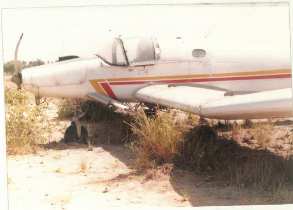
AIRCRAFT AT SITE EVIDENCE: PROP DAMAGE
