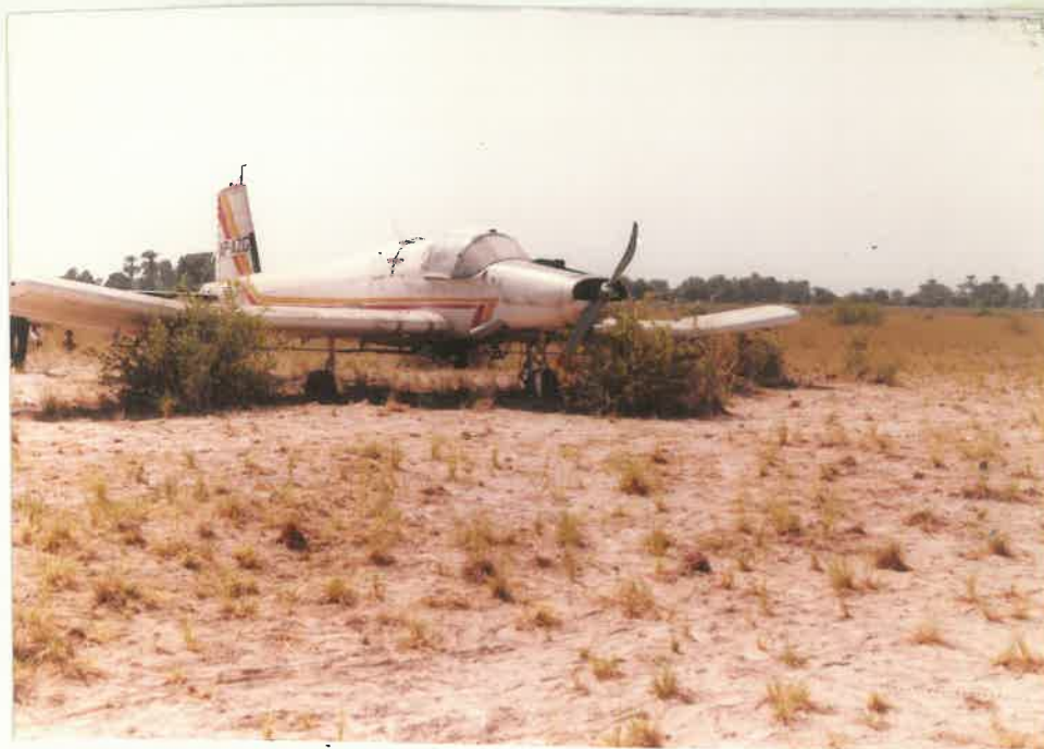
AIRCRAFT AT SITE EVIDENCE: BUMPY SANDY FIELD & PROP DAMAGE
