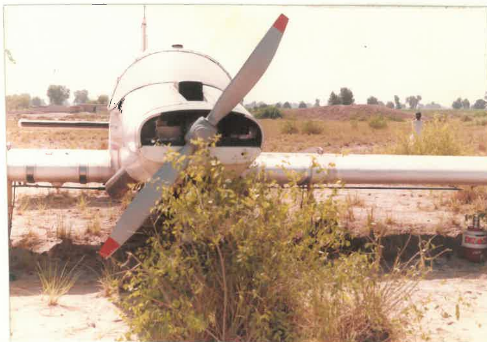
AIRCRAFT AT SITE EVIDENCE: BACK GROUND OF LANDING FIELD & PROP DAMAGE
