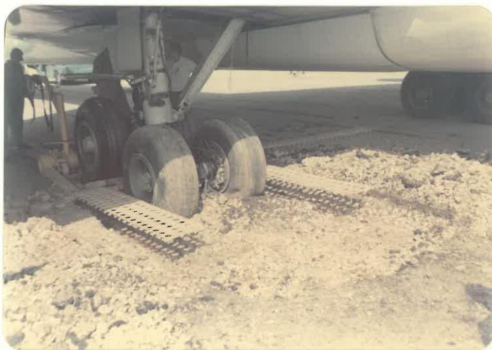
PORT MAIN LANDING GEAR SUNK INTO GROUND APPROX. 6" TO 8"
