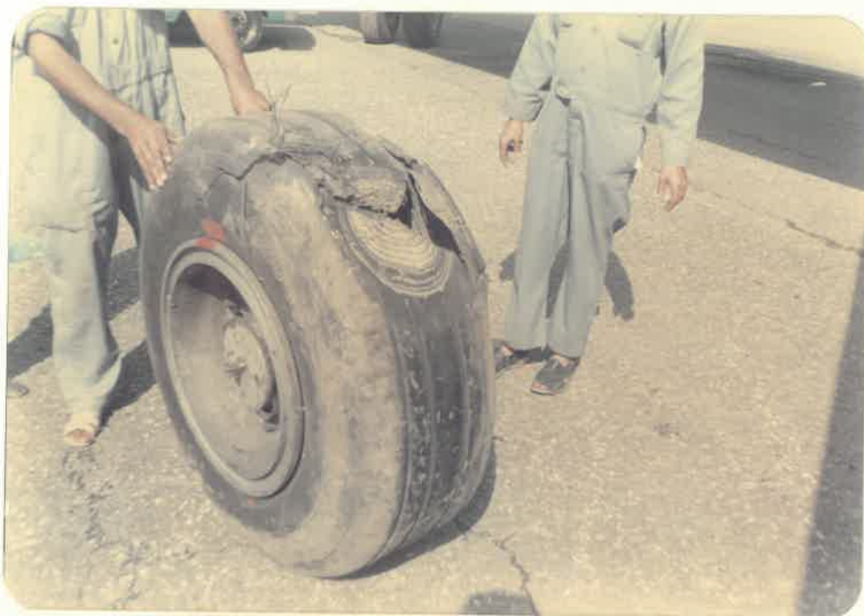
FORWARD NO.1 TYRE ALREADY REMOVED ON 17.10.90 SHOWING DAMAGE DUE TO EXCESSIVE BRAKING.
