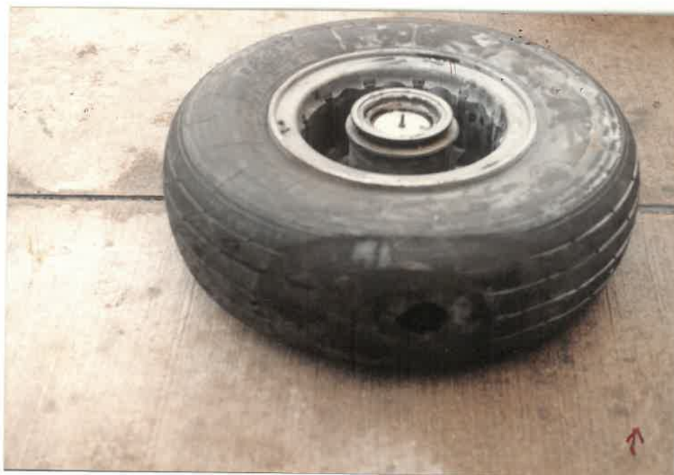
REAR TYRE : KNOT IN THE WOOD TYPE EVIDENCE (ANOTHER VIEW)
