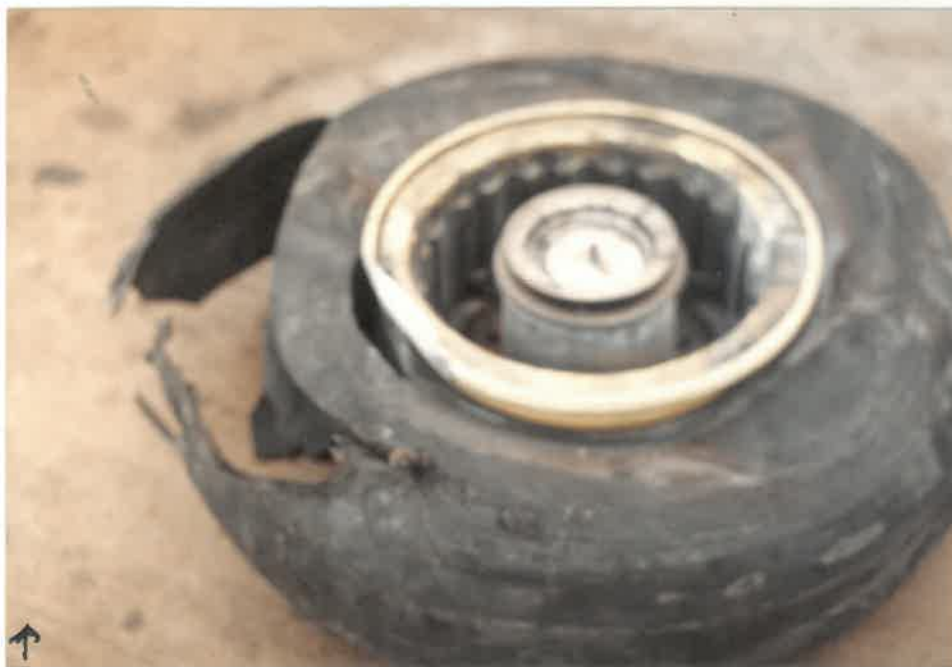
FORWARD WHEEL NOTE: NOTE LATERAL RUBBING MARKS
