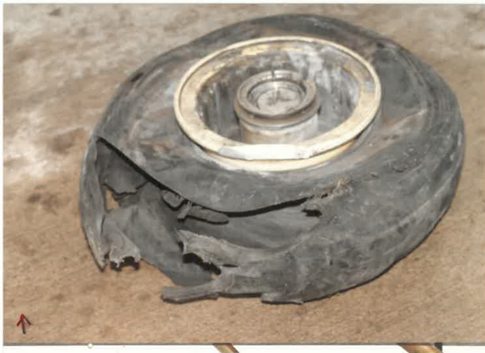
LEFT MLG FORWARD WHEEL NOTE: * LATERAL RUBBING MARKS * DISFIGUREMENT
