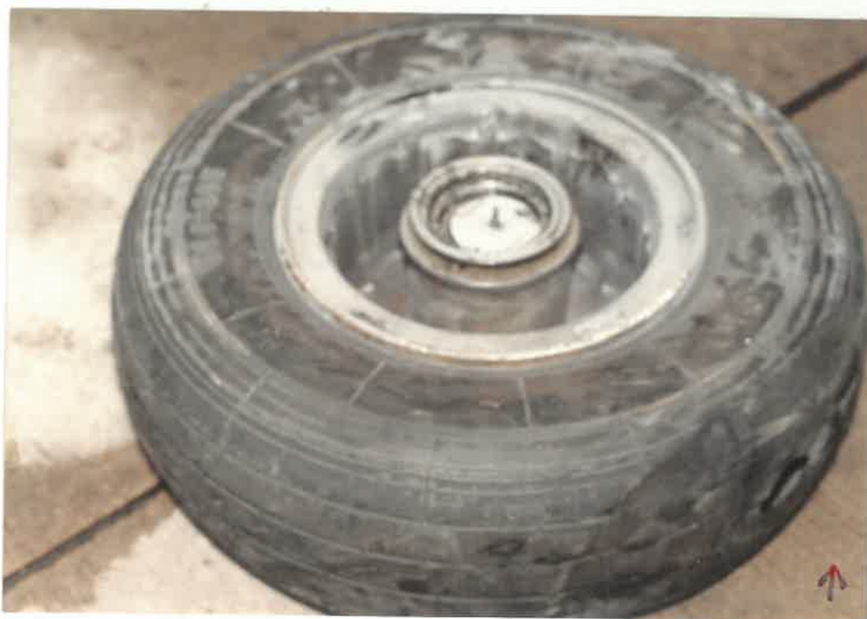
REAR TYRE : RUBBING MARK DUE TO WHEEL LOCK NOTE - KNOT IN THE WOOD TYPE EVIDENCE
