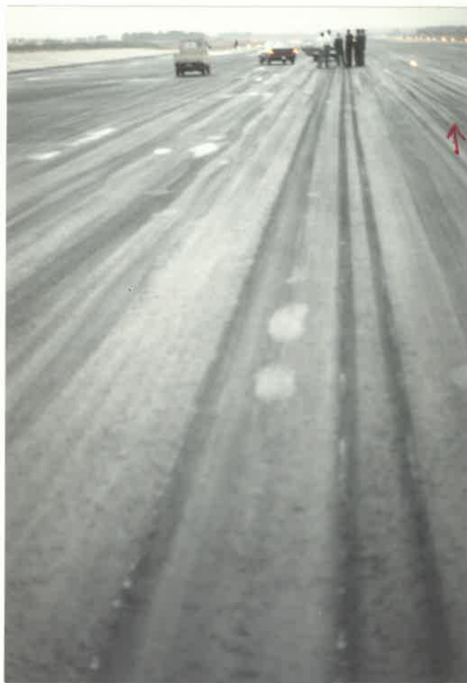
LEFT MLG TYRE MARKS BETWEEN 4000 TO 5000 FEET FROM THE STOPPING POINT OF A/C
