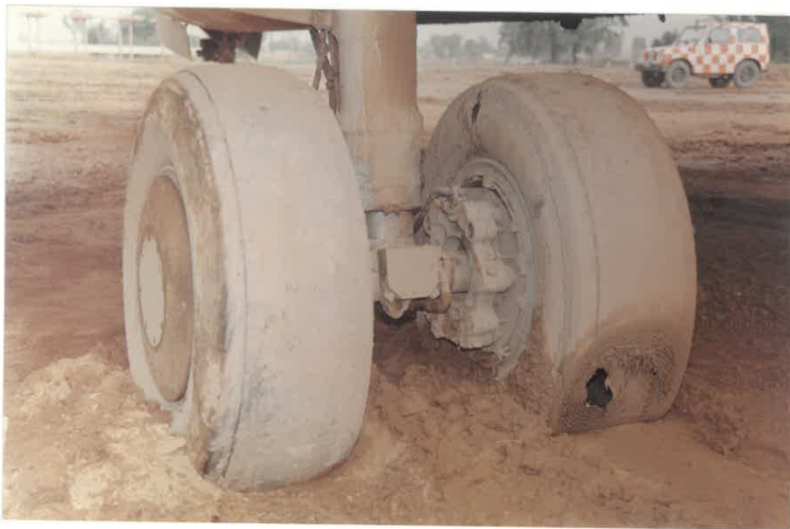
LEFT MAIN GEAR TYRES VIEWED FROM REAR OF AIRCRAFT (NO.2 TYRE WITH A FLAT SPOT BURST & NO.1 TYRE BALD)
