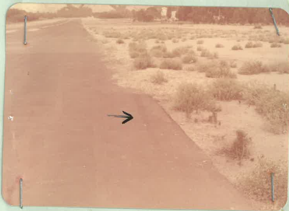
TYRE MARKS SHOWING LEFT HAND MAIN LANDING GEAR DEPARTING THE RUNWAY SURFACE. NOTE THE CONTROL TOWER AND THE FIRE STATION BUILDINGS ON RIGHT OF THE RUNWAY.
