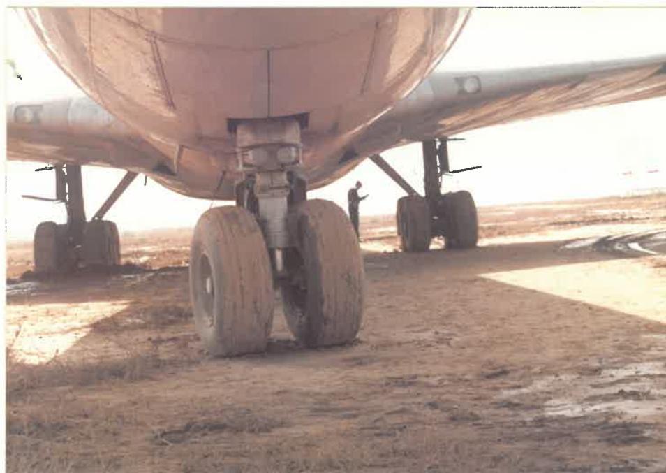
RIGHT WHEEL SUNK IN THE SOGGY/KATCHA AREA - LEFT MAIN WHEEL AND NOSE WHEEL ON A COMPACTED KATCHA GROUND
