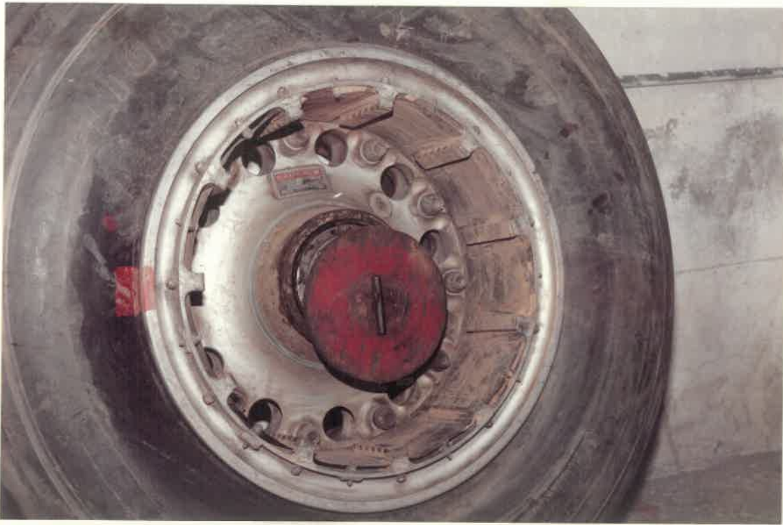
TYRE CREEP MARKS STILL IN PLACE
