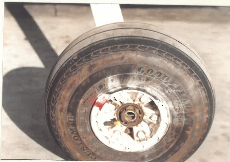
RIGHT MAIN WHEEL HUB CRACKED
