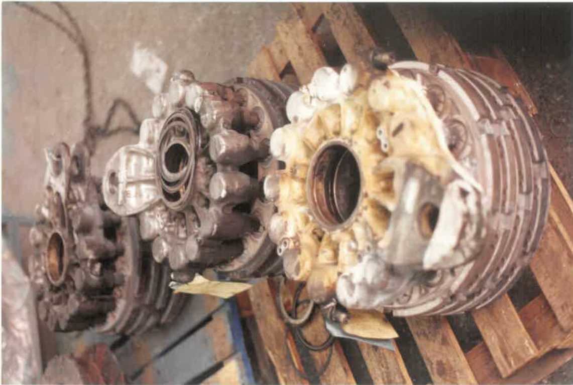
BRAKE ASSEMBLIES SHOWING HEAT EFFECT
