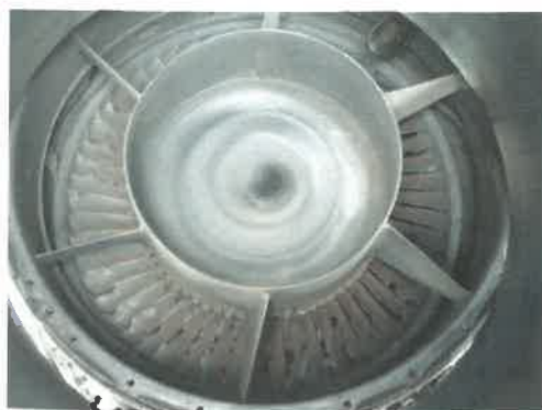
Power and free turbine damage, pictured on post flight
