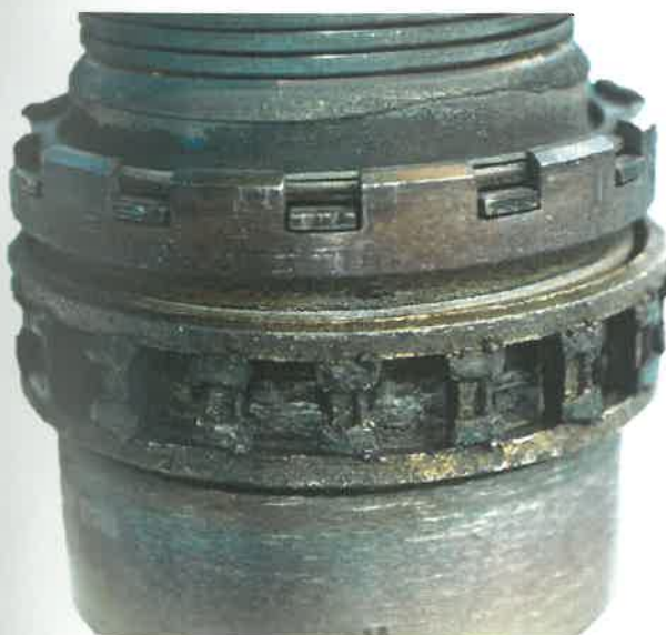
Fig.7. Oxide deposits on the inner race of roller bearing.
