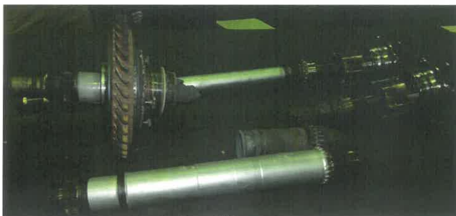
Comparison of PT shaft and LP shaft damage with new parts
