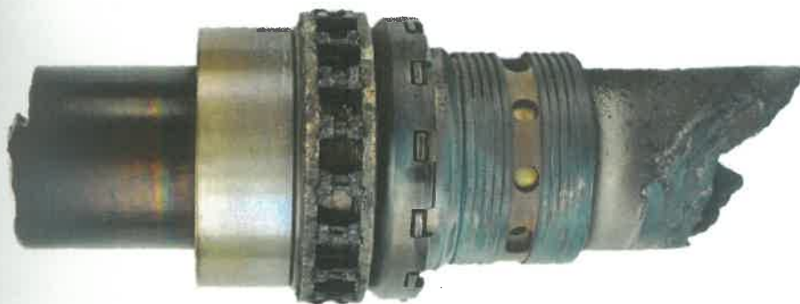
Fig. 6. Inner race of roller bearing attached with left over portion of PT shaft.
