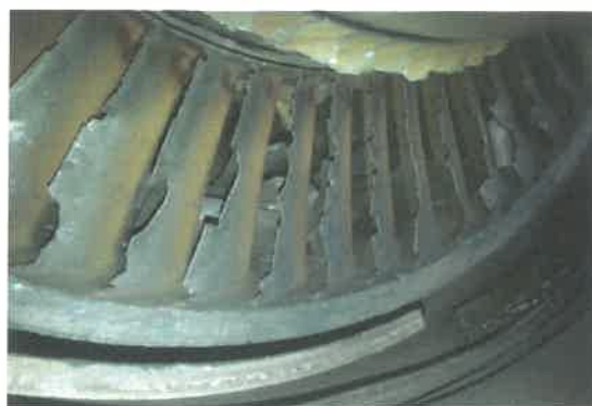
Power and free turbine damage, pictured on post flight
