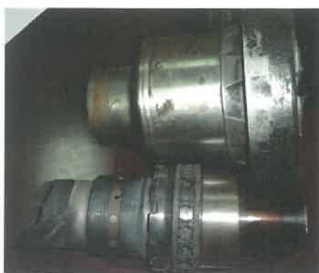
No. 2 Bearing and its housing
