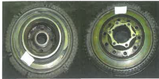
Power turbine 1 and 2 (Blades removed for inspection)
