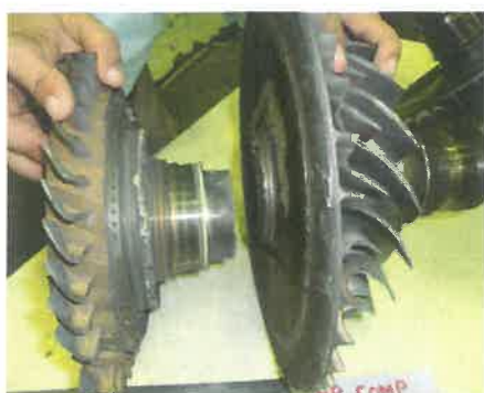
HP compressor and HP turbine and HP shaft damage
