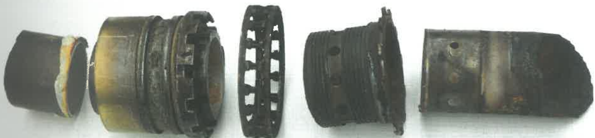
Fig. 10. Disassembled inner race of roller bearing.
