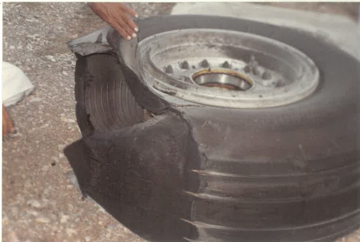
TYPICAL TYRE & RIM AFTER THE INCIDENT. NOTE: THE DRAG MARK ON THE RIM OUTER SURFACE
