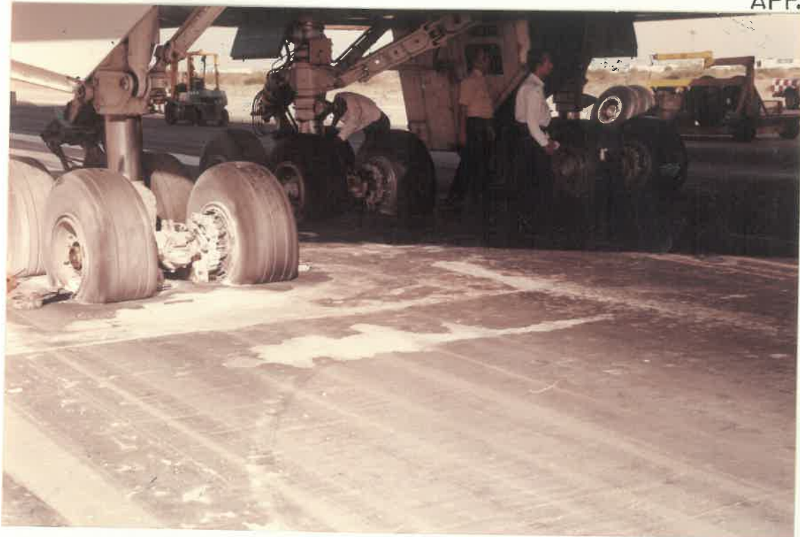
PHOTO TAKEN AFTER LANDING LEFT BODY GEAR & WING GEARS TYRES BURST
