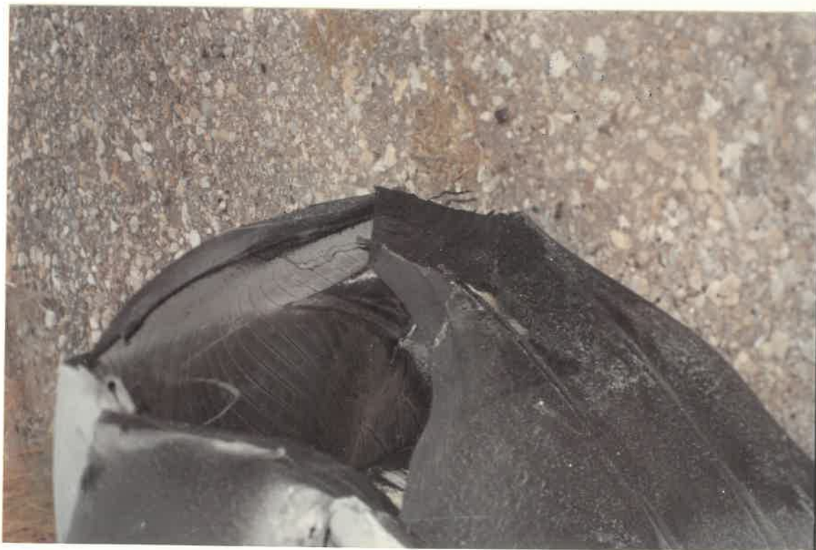
TYPICAL TYRE BURST SURFACE
