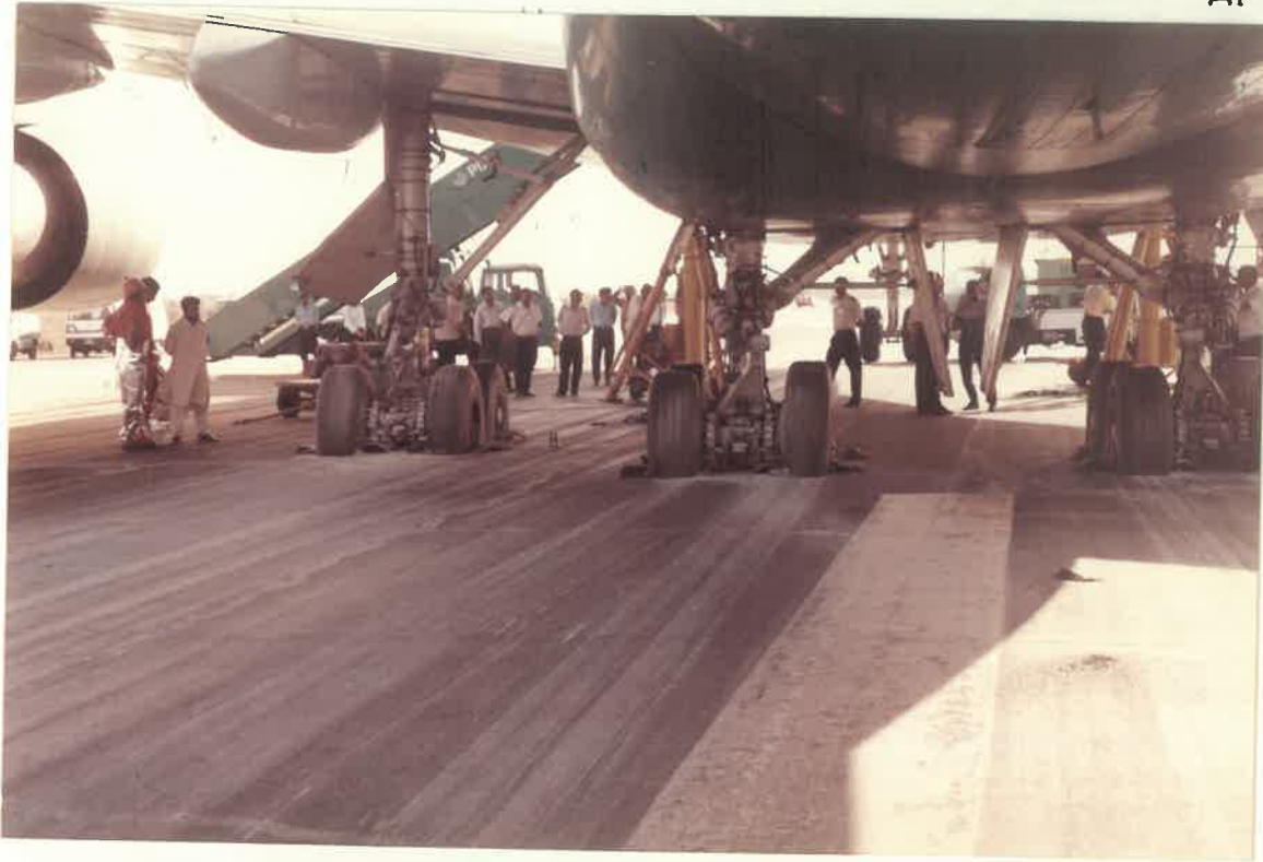
PHOTO TAKEN AFTER LANDING LEFT BODY GEAR & WING GEARS TYRES BURST
