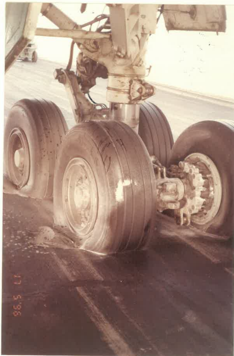
LT. WING GEAR WING GEAR TYRES BURST
