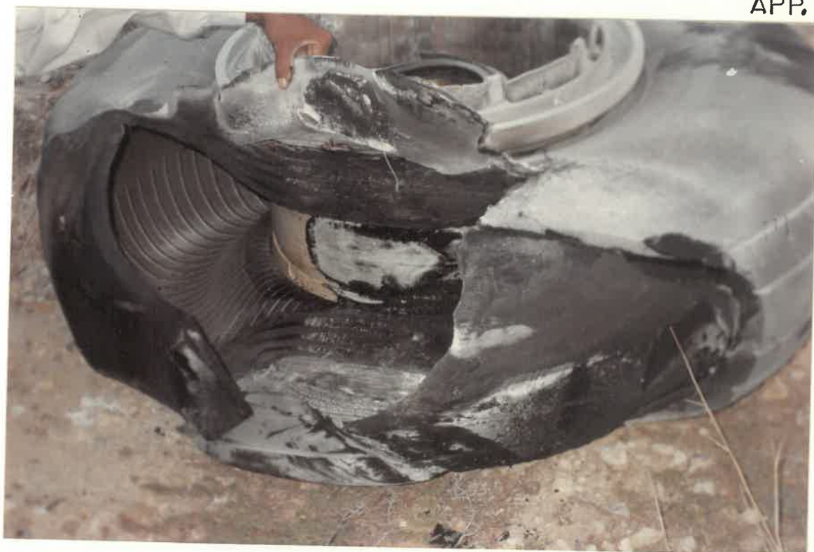
TYPICAL TYRE BURST SURFACE
