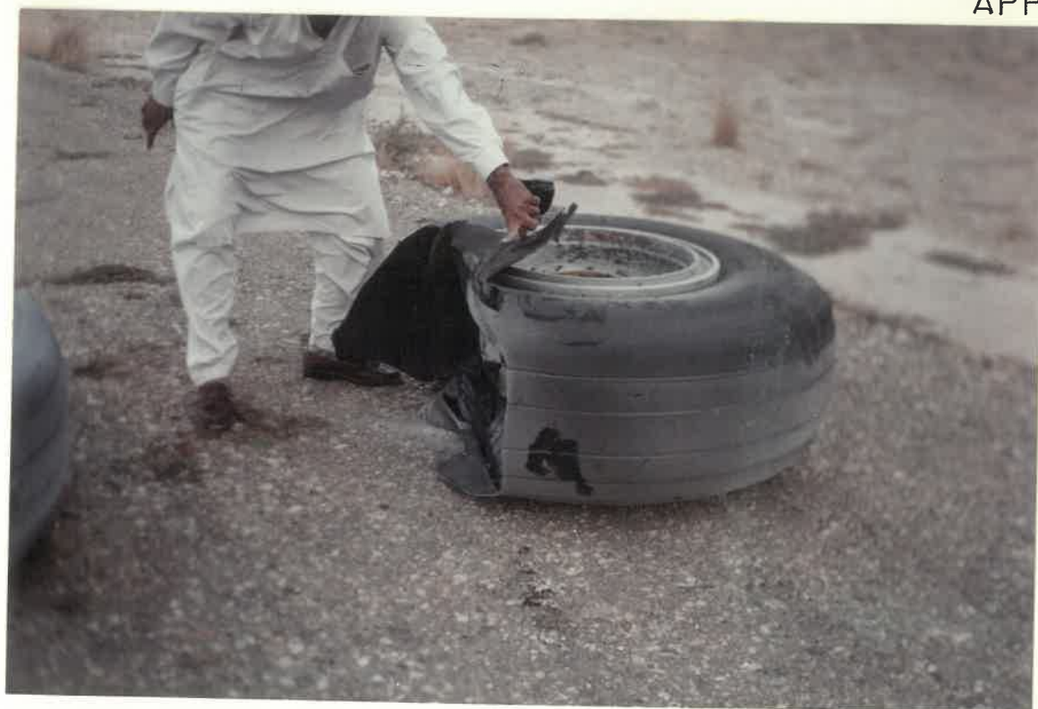
TYPICAL TYRE BURST SURFACE
