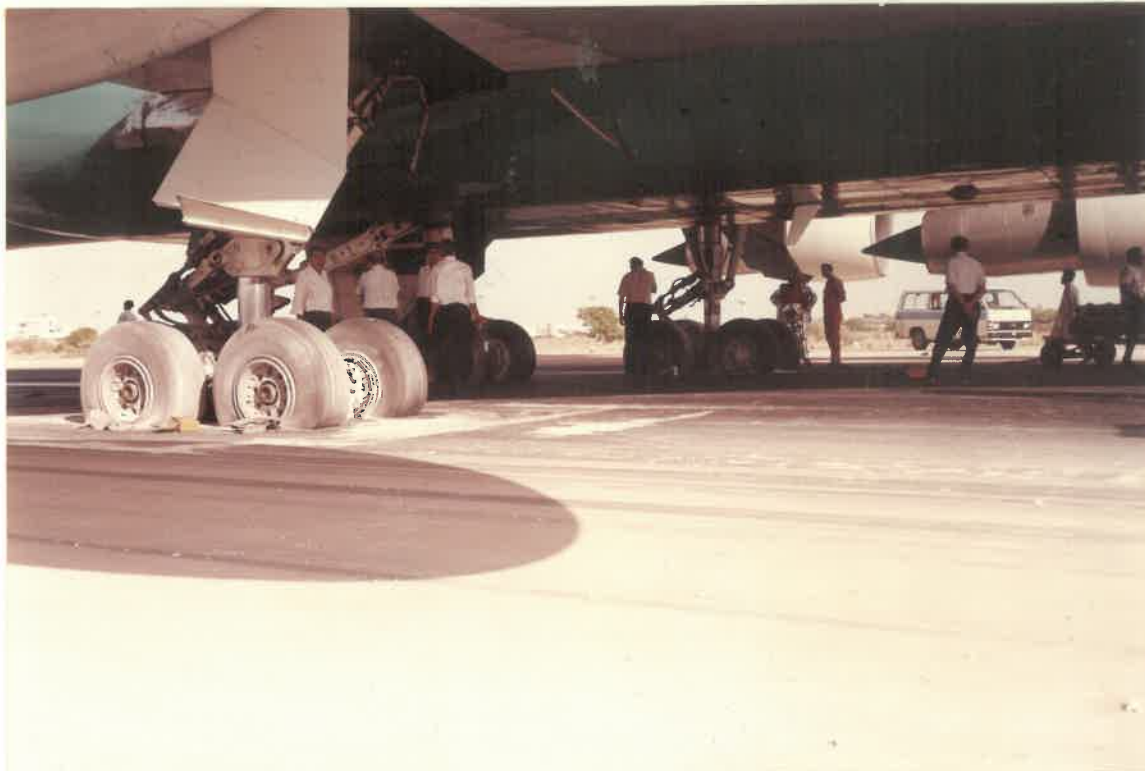
ANOTHER VIEW OF LEFT WING GEAR TYRES BURST
