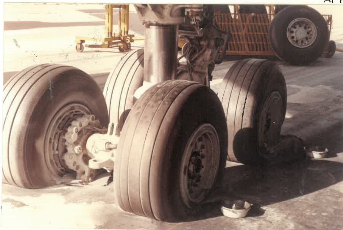
ALL TYRES BURST WING GEAR
