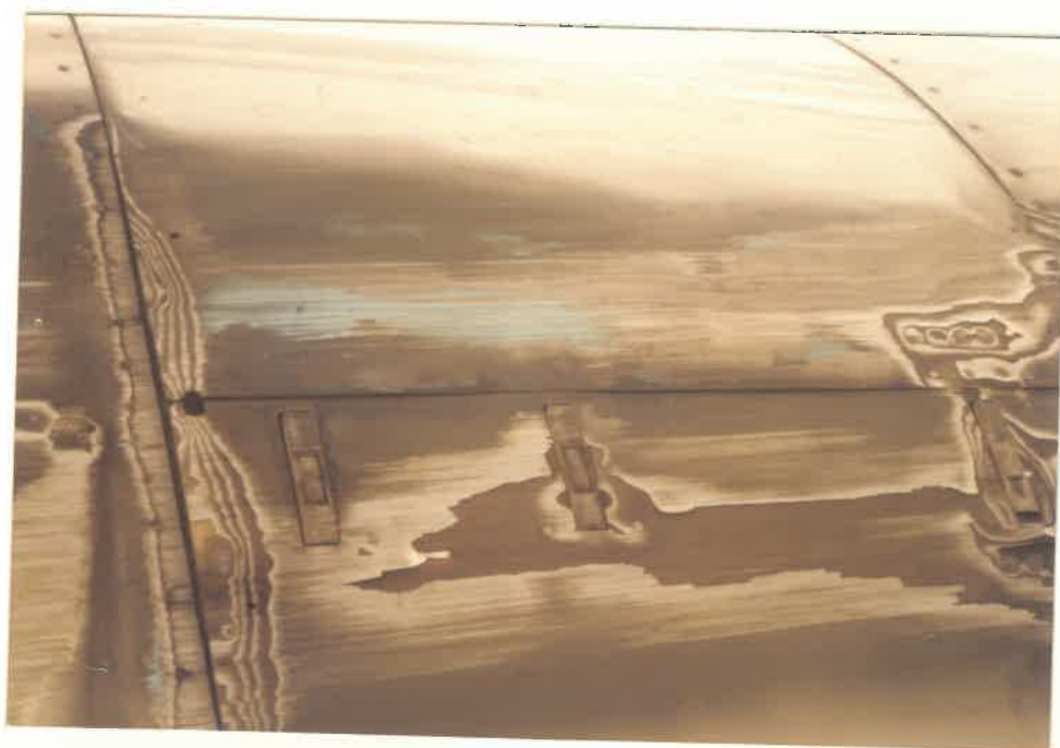
UNDER SURFACE SCRUB MARKS ON NO.1 ENGINE
