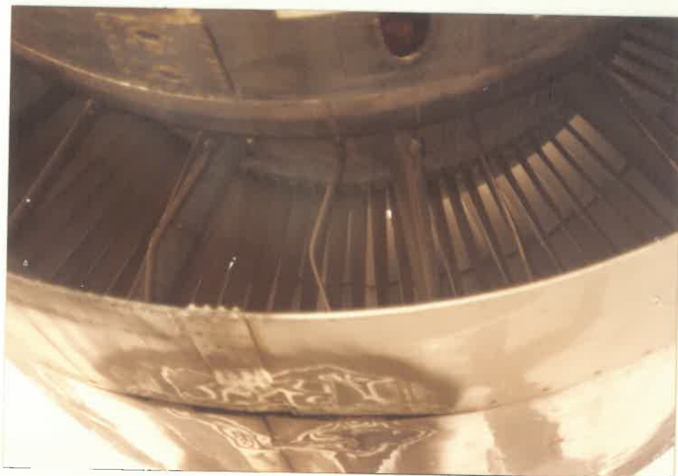
21 UNDER SURFACE DAMAGE OF NO.1 ENGINE
