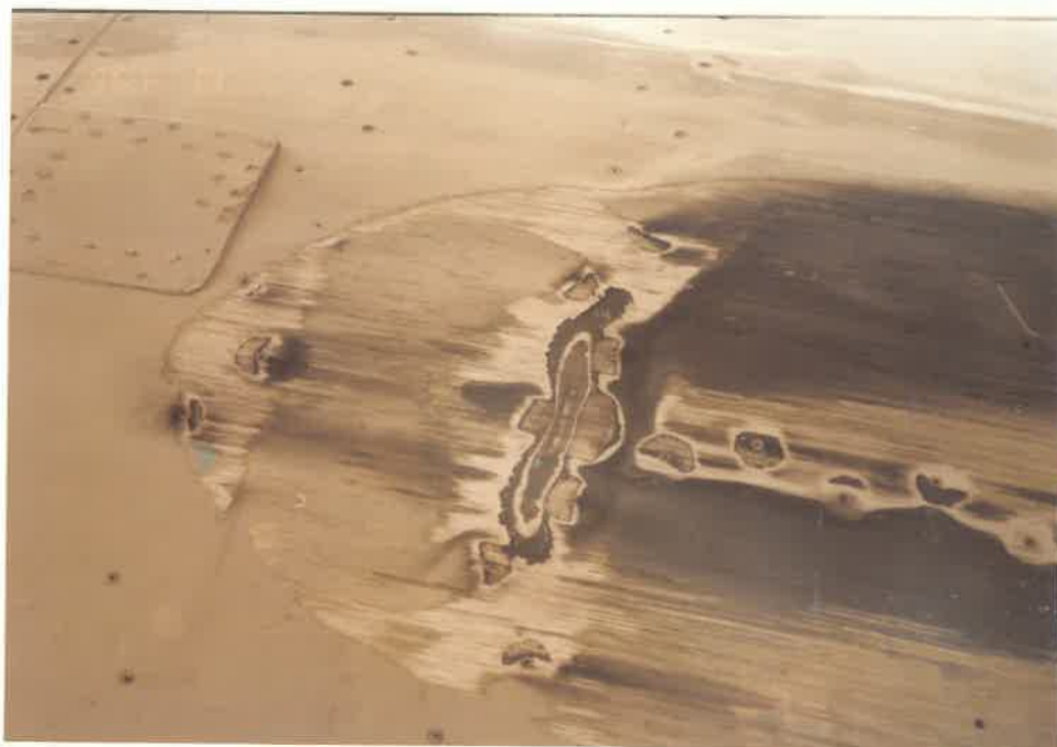
UNDER SURFACE DAMAGE OF NO.1 ENGINE
