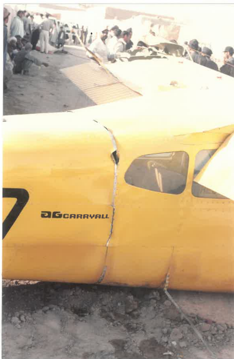
DAMAGED AIRCRAFT WITH DETACHED PESTICIDE TANK
