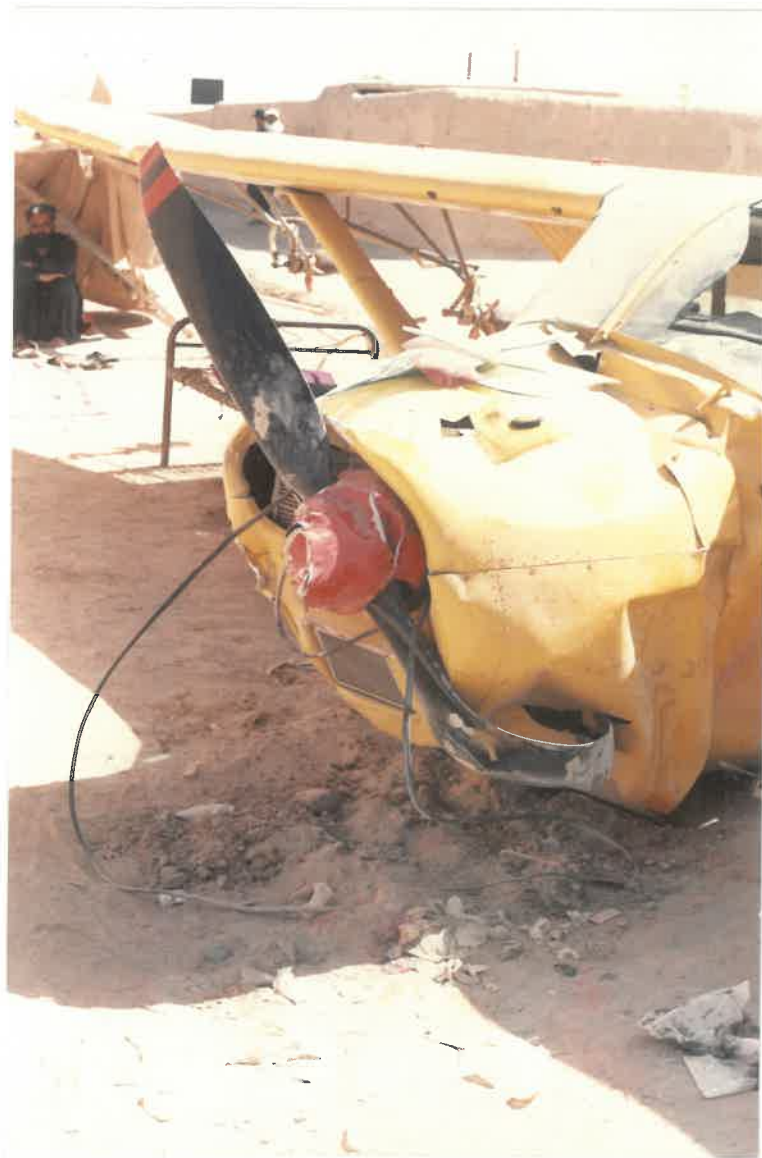
ELECTRIC WIRE WRAPPED AROUND THE PROP. INDICATIVE OF NOSE IMPACTING FIRST AT ABOUT 45/50° AND BEFORE THE TAIL COMING DOWN.
