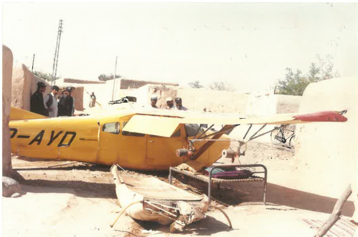
DAMAGED AIRCRAFT WITH DETACHED PESTICIDE TANK
