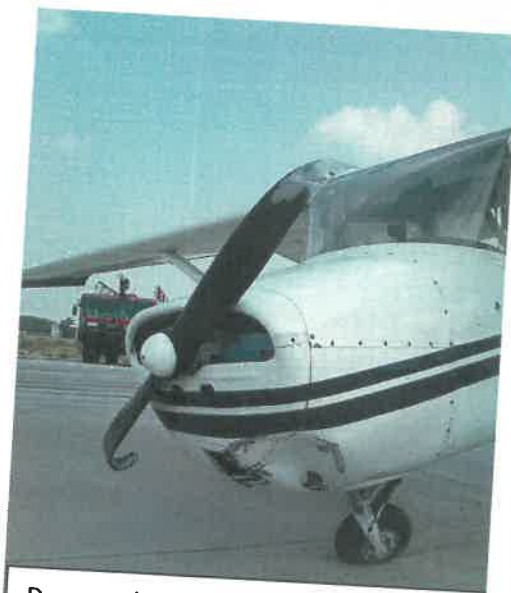
Damaged Propeller and Nose area
