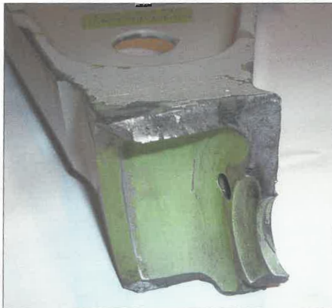
PHOTO 5 UPPER TORSION LINK - AS RECEIVED
