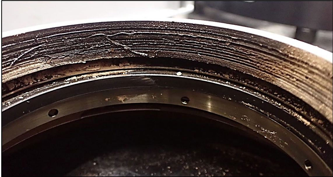
Figure 12 Bearing No.1 Cover close-up view
