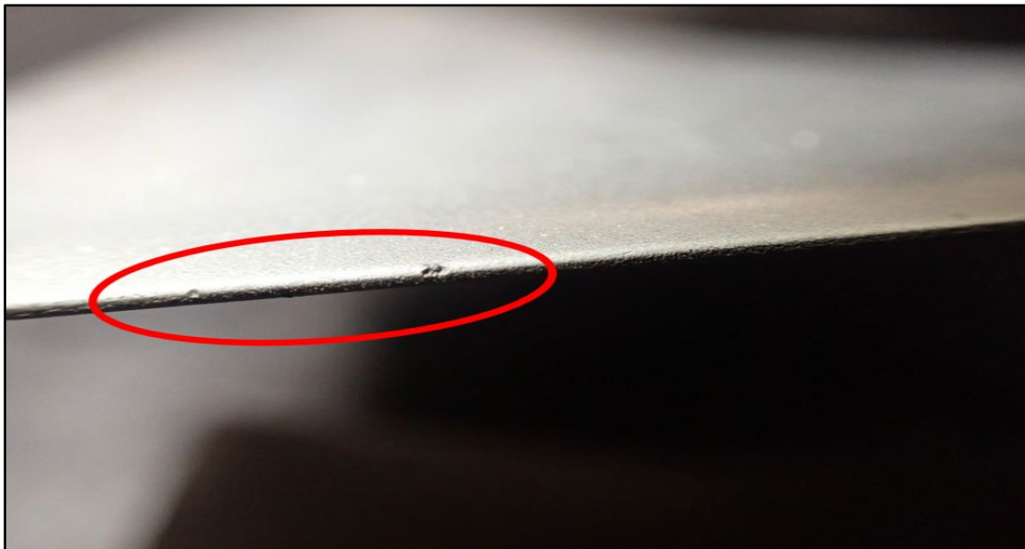
Figure 2 Nick Marks on LP Rotor Balancing Assembly (Fan)
