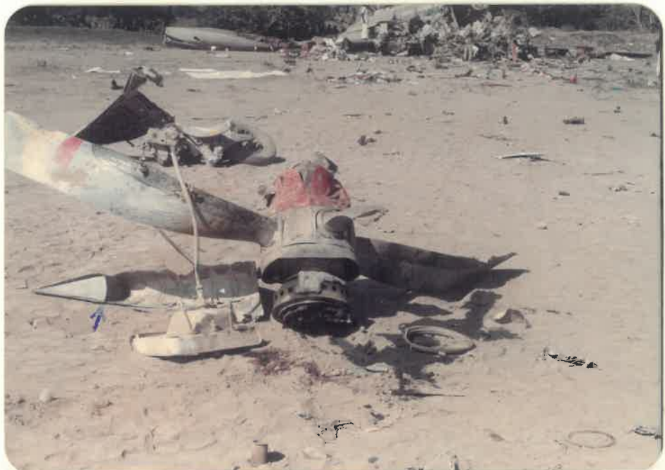
VIEW OF LEFT ENGINE PROPELLER. ENGINE WAS DEVELOPING POWER WHEN BLADES CONTACTED THE GROUND AFTER SECOND IMPACT AS THE AIRCRAFT WAS NOSING OVER.
