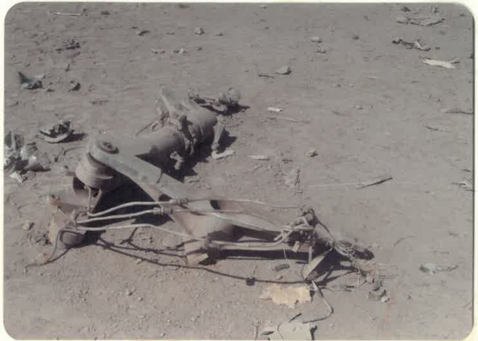
STARBOARD MAIN LANDING GEAR STRUT WHICH BROKE OFF ON INITIAL IMPACT.
