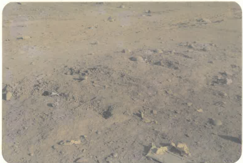
SLASH MARKS MADE BY LEFT PROPELLER BLADES ALL FOUR BLADES STRUCK THE GROUND.
