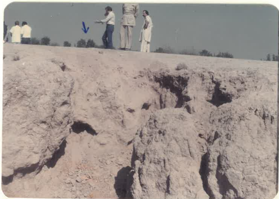
ARROW POINTS TO MARKS MADE BY THE REAR UNDER SURFACE OF THE FUSELAGE. TOILET DRAIN WAS FOUND AT THIS POINT.
