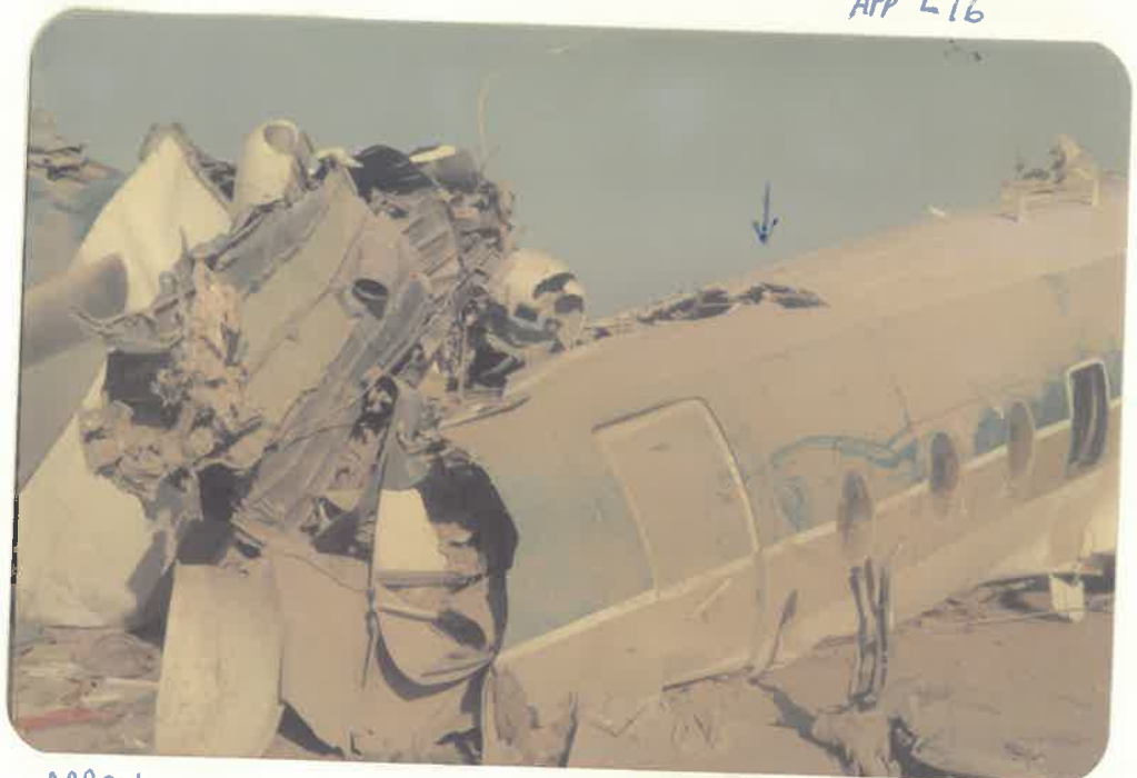
ARROW INDICATES DAMAGE TO THE REAR UNDERSURFACE OF THE FUSELAGE. THIS DAMAGE PROCEEDS BACK TO A POINT JUST AHEAD OF THE EMPENNAGE. THE FUSELAGE IS INVERTED WHEREAS THE EMPENNAGE IS FIN UP. IT WAS TURNED THROUGH 180 DEGREES.
