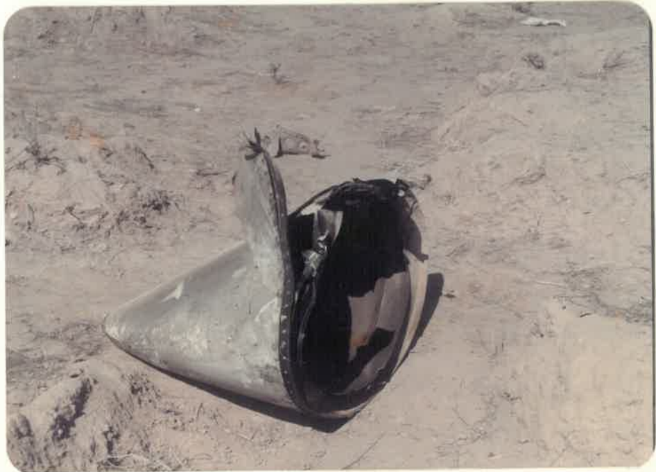
TAIL CONE OF RIGHT ENGINE NACELLE WHICH WAS RIPPED OFF WHEN STRUCK BY SOME PART OF THE RIGHT MAIN LANDING GEAR WHICH BROKE OFF ON FIRST IMPACT.
