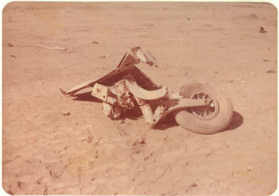
VIEW OF NOSE LANDING GEAR WHICH WAS DAMAGE AT SECOND IMPACT. NOSE GEAR DAMAGE INDICATES IT WAS DOWN AND LOCKED AT TIME OF THIS IMPACT
