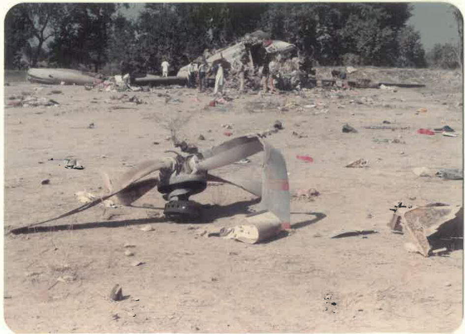
VIEW OF RIGHT ENGINE PROPELLER. ENGINE WAS DEVELOPING POWER WHEN BLADES CONTACTED THE GROUND AFTER SECOND IMPACT AS THE AIRCRAFT WAS NOSING OVER. MAIN WRECKAGE CAN BE SEEN IN THE BACKGROUND.
