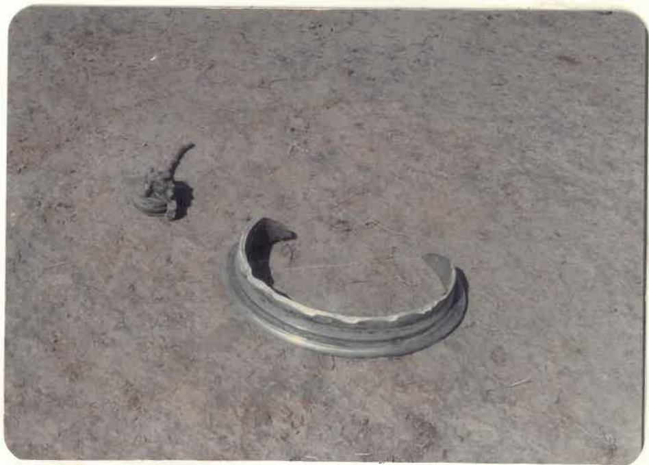
RIM OF THE RIGHT STARBOARD MAIN WHEEL. FAILURE OCCURRED TO OUTBOARD WHEEL ON INITIAL IMPACT.
