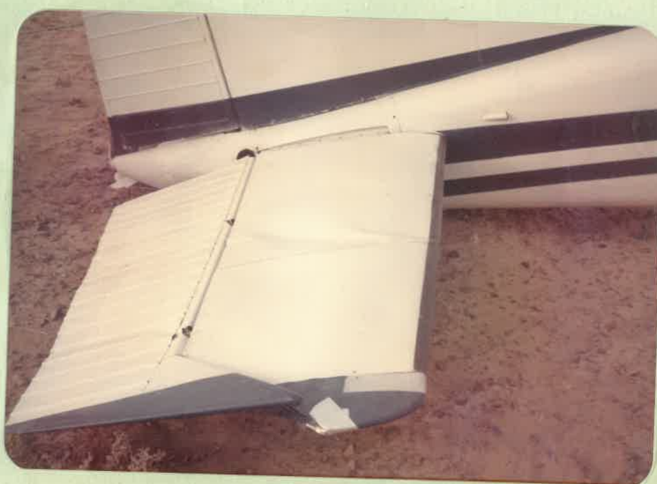
RIGHT SIDE TAIL SECTION DAMAGED AND BENT
