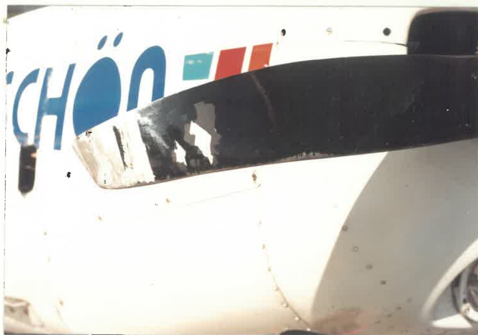
DAMAGED PROPELLER BLADE ANOTHER VIEW
