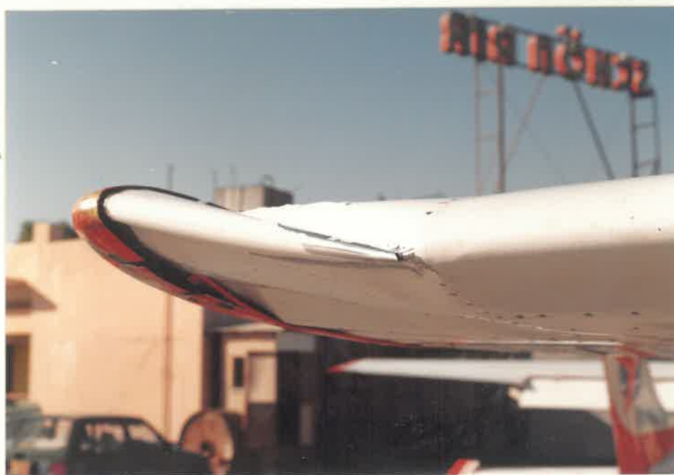
RIGHT WING TWISTED AND BUCKLED
