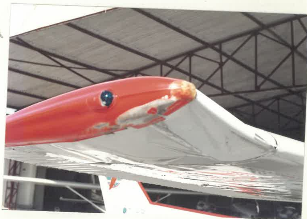
RIGHT WING TIP TWISTED
