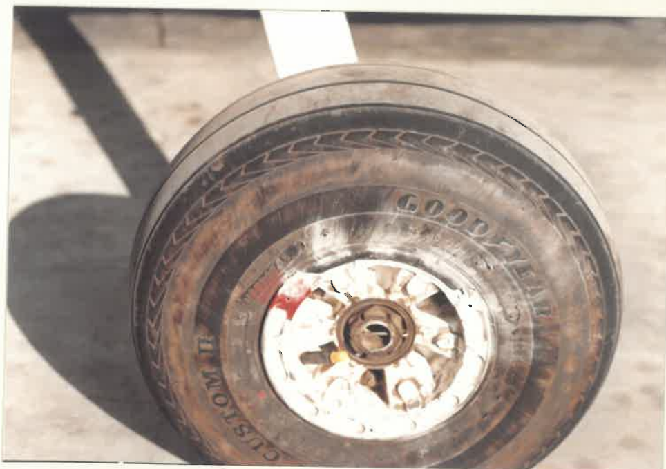
RIGHT MAIN WHEEL HUB CRACKED
