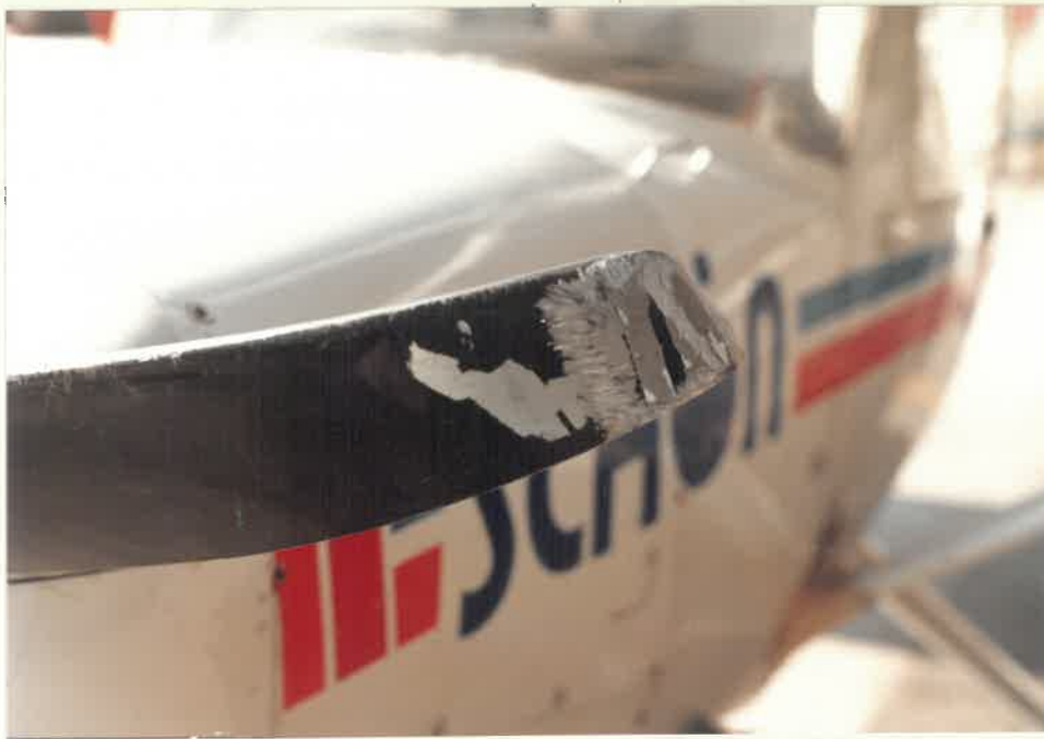
DAMAGED PROPELLER BLADE
