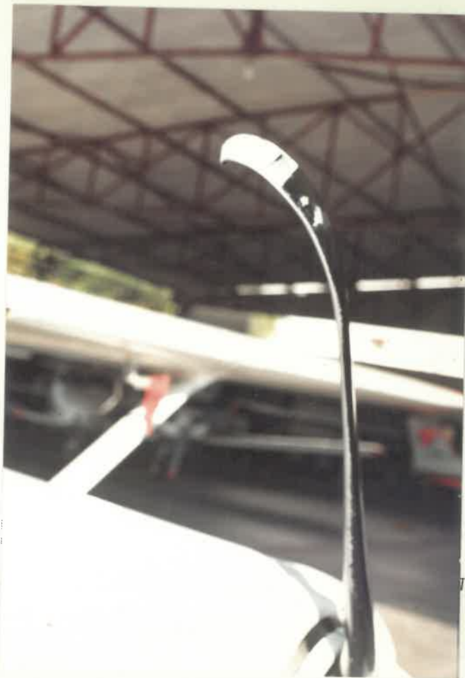
DAMAGE PROPELLER BLADE ANOTHER VIEW
