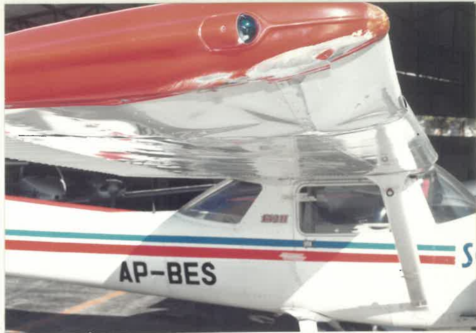
RIGHT WING DAMAGE
