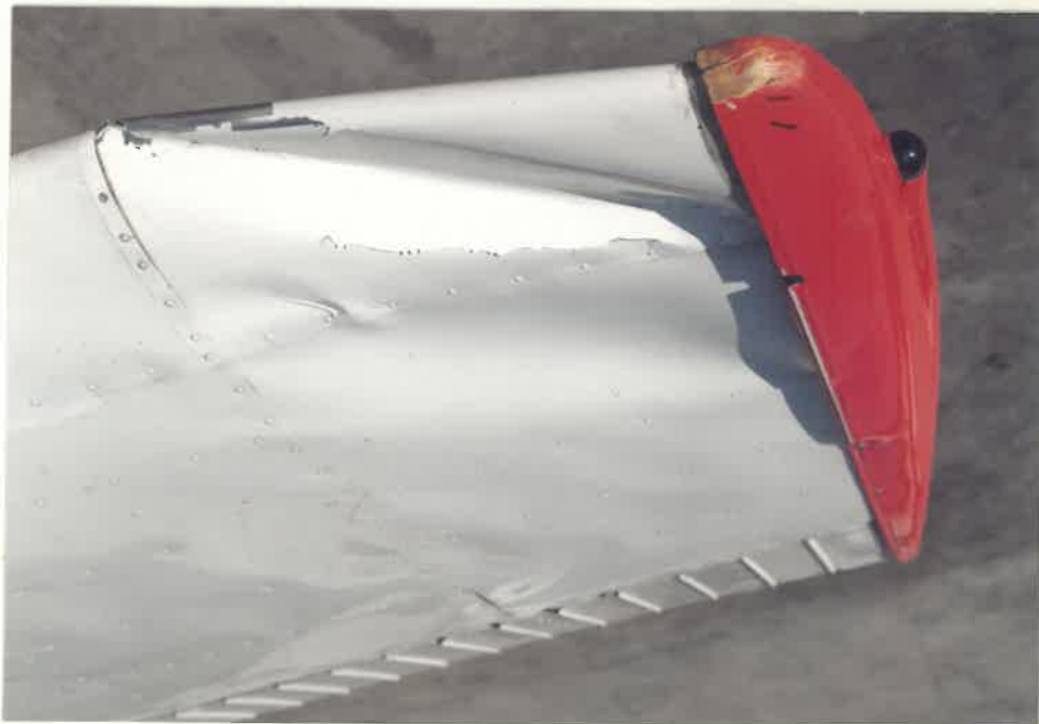
RIGHT WING TIP DAMAGE
