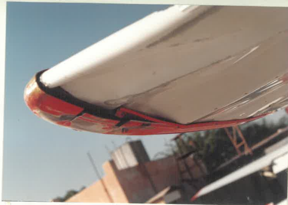
RIGHT WING UNDER SURFACE SCRATCHED AND BUCKLED
