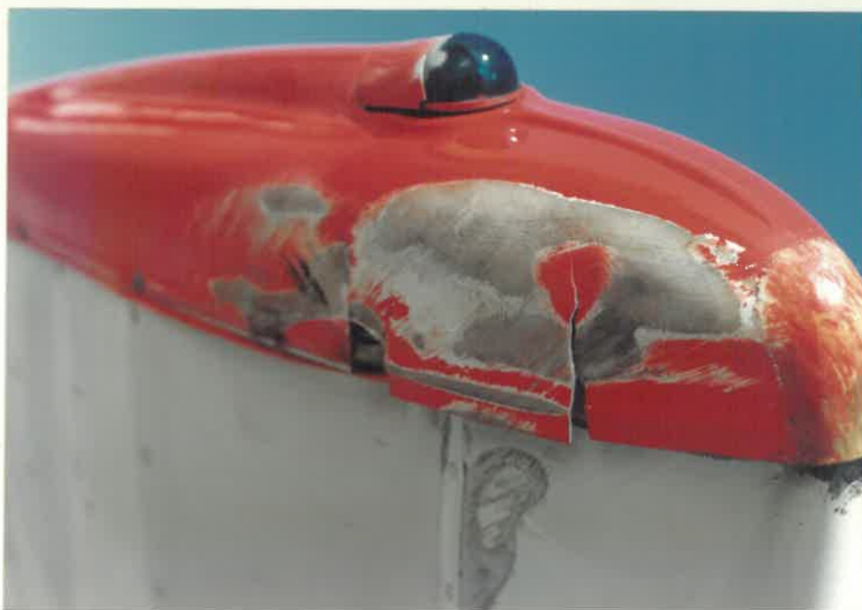
RIGHT WING TIP DAMAGE ANOTHER VIEW
