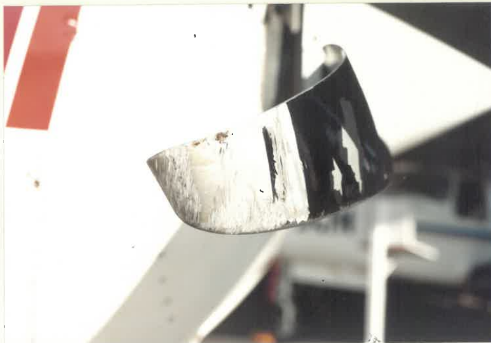
DAMAGED PROPELLER BLADE
