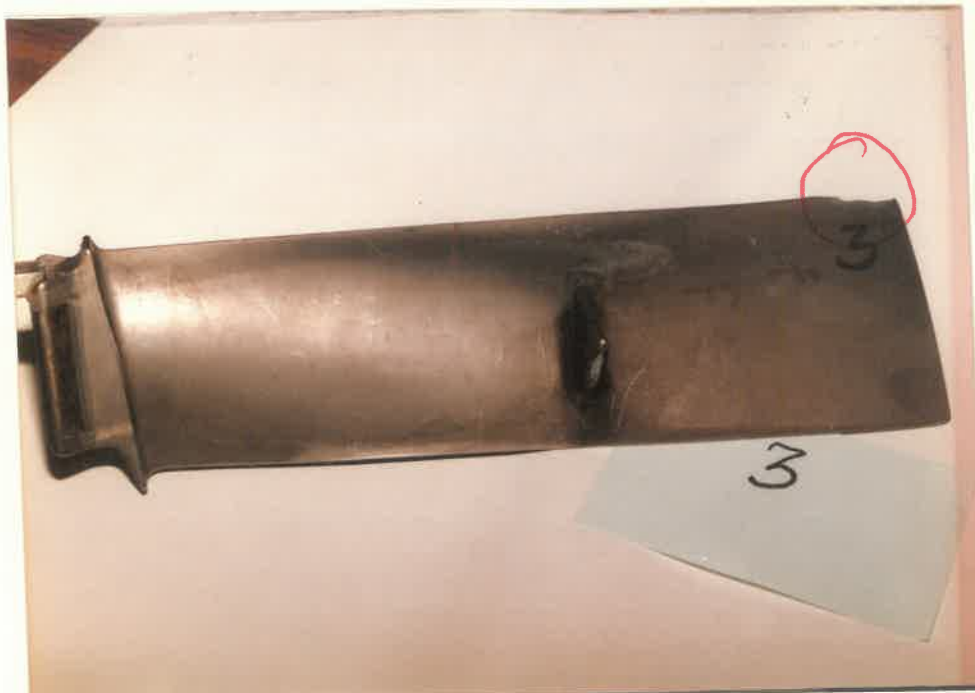
ANOTHER 1ST STAGE COMP BLADE DAMAGED
