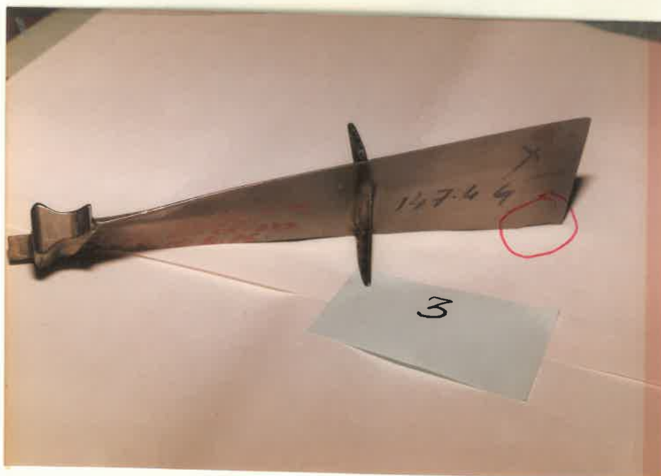
ANOTHER 1ST STAGE COMP BLADE DAMAGED
