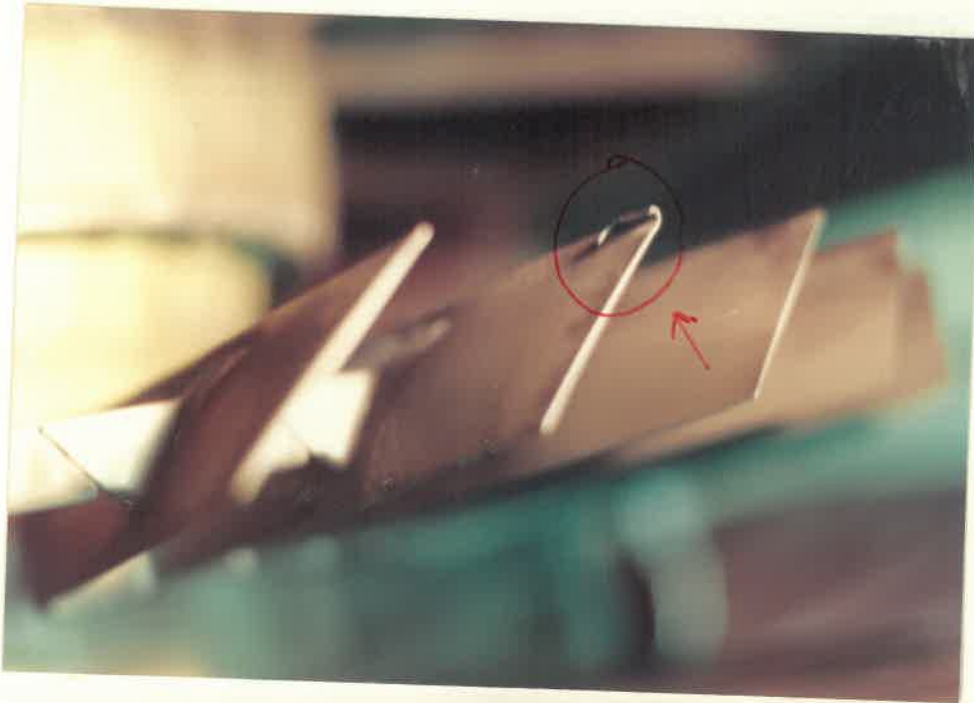
EVIDENCE OF BLADE DAMAGE 1ST STAGE COMP BLADE
