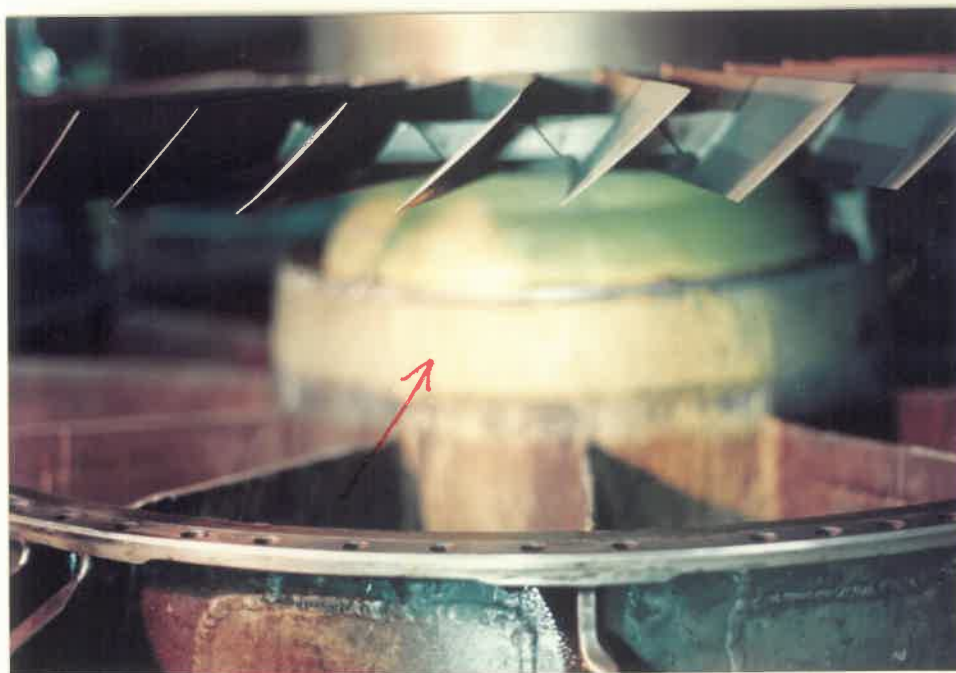
ANOTHER VIEW OF EVIDENCE OF BIRD INJECTION IN THE ENGINE IN TAKE
