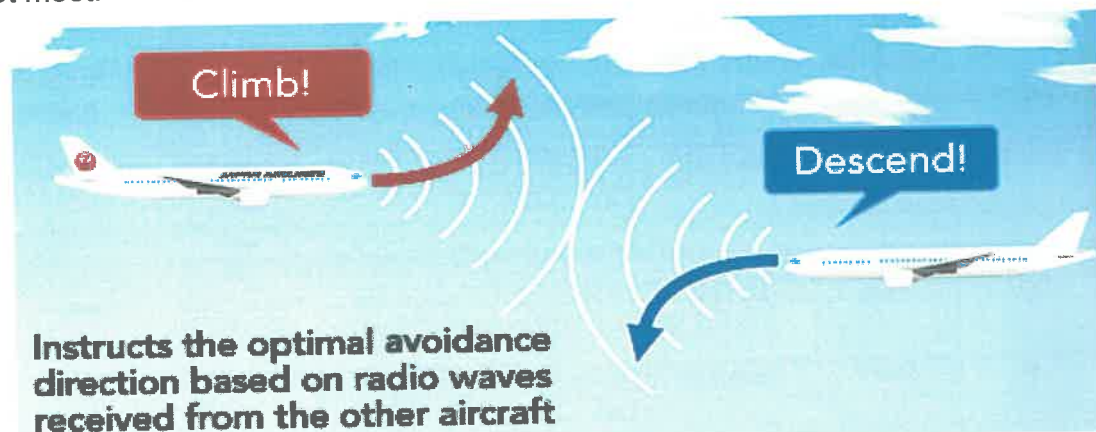
Figure 2 TCAS Working Principle
