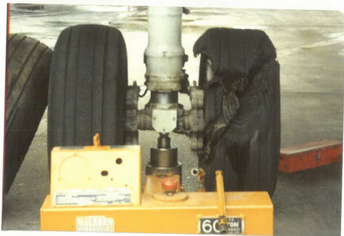
Left main landing gear wheels with inboard tyre burst and scuff.
