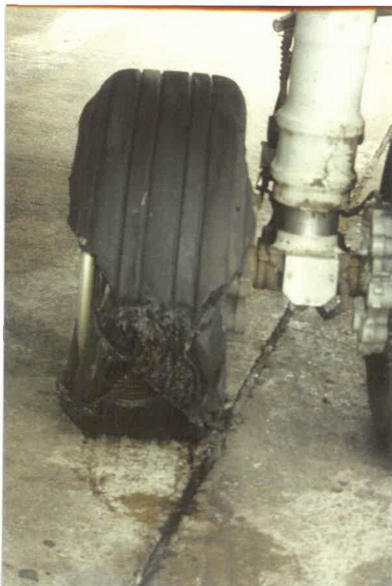
Right main landing gear inboard tyre burst (close up).
