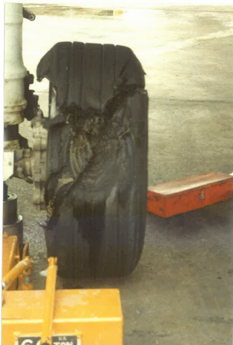
Left main landing gear inboard tyre burst (close up).
