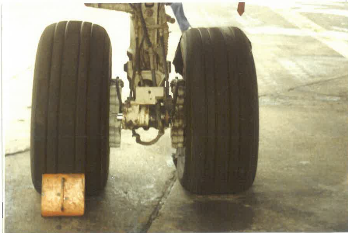
Left main landing gear wheels with inboard tyre burst.
