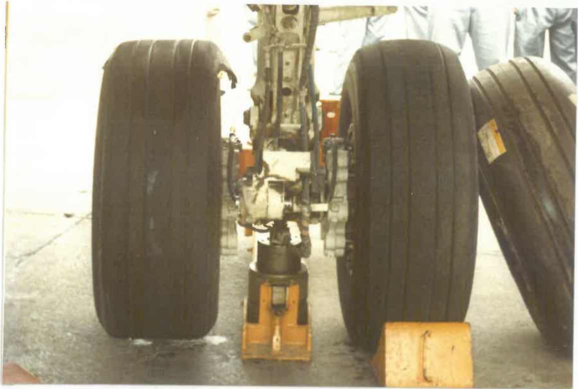
Right main landing gear wheels with inboard tyre burst.
