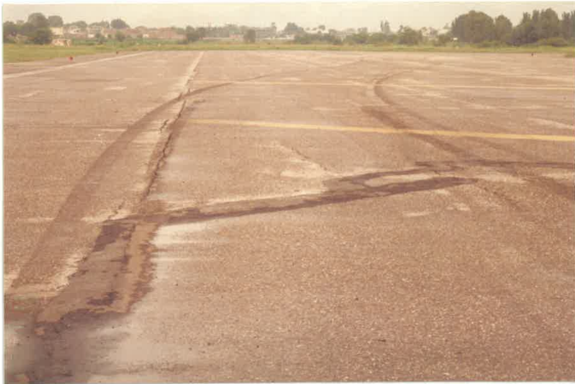
Both main landing gears wheels (both inner and outer) marks on over-run area.
