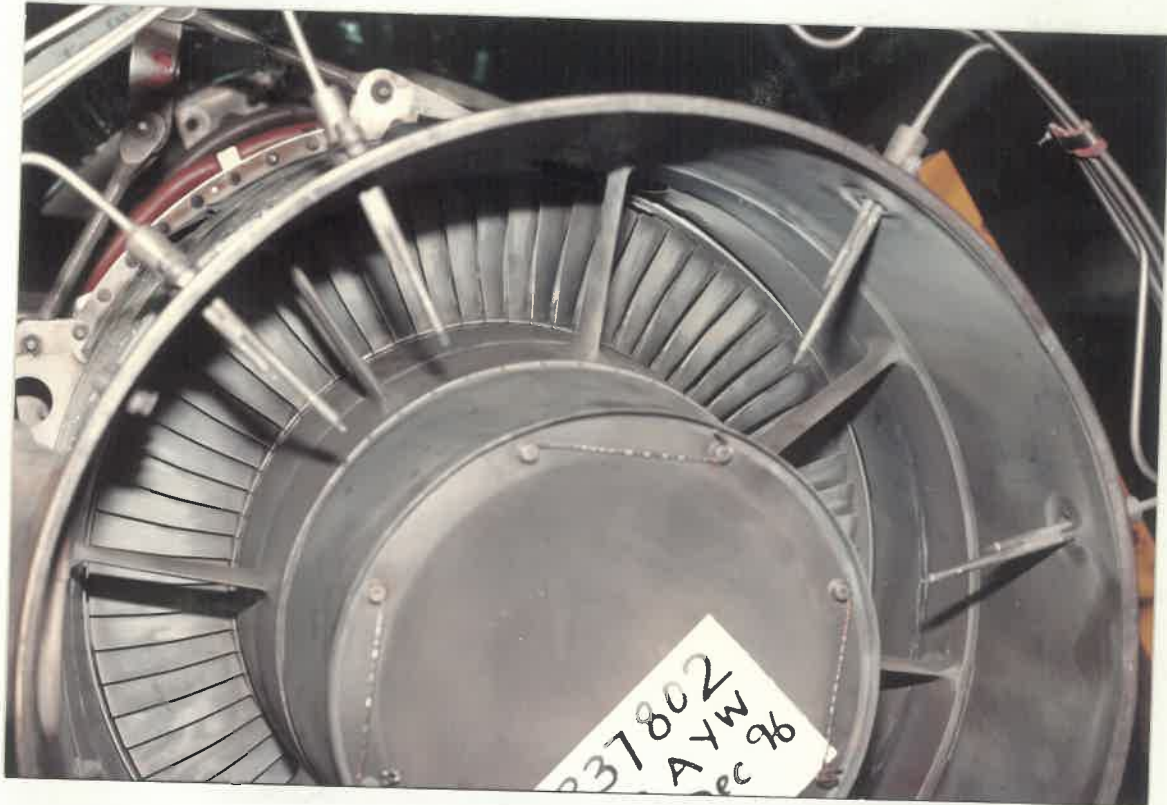
EVIDENCE OF OVERHEAT IN THE APU
