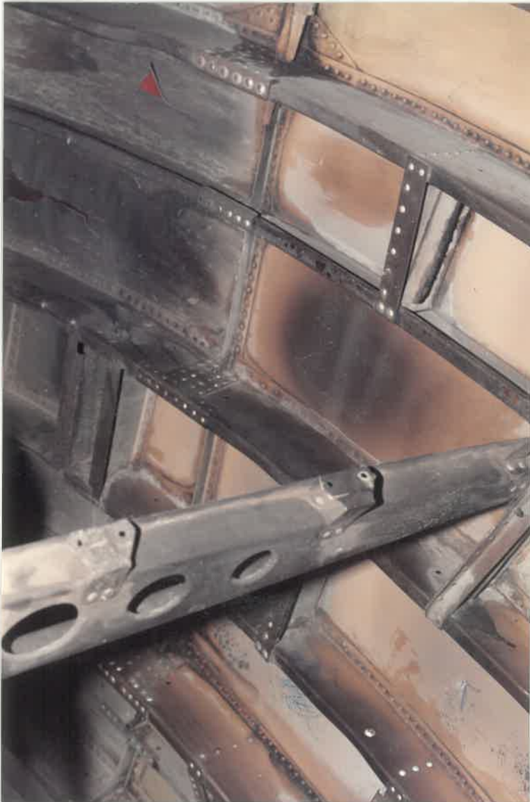
INSIDE VIEW OF DAMAGE CAUSED IN THE TAIL SECTION
