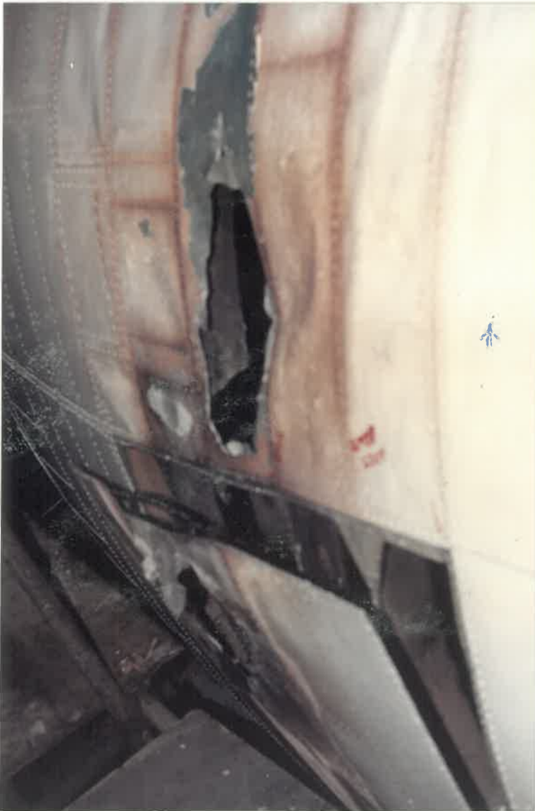
EVIDENCE OF BURNING AND BUCKLING OF TAIL SKIN - ANOTHER VIEW
