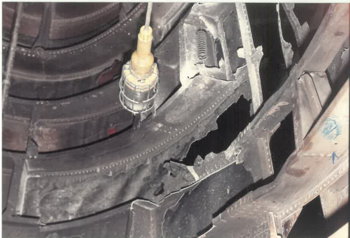
FIRE DAMAGE TO TAIL SECTION INSIDE VIEW
