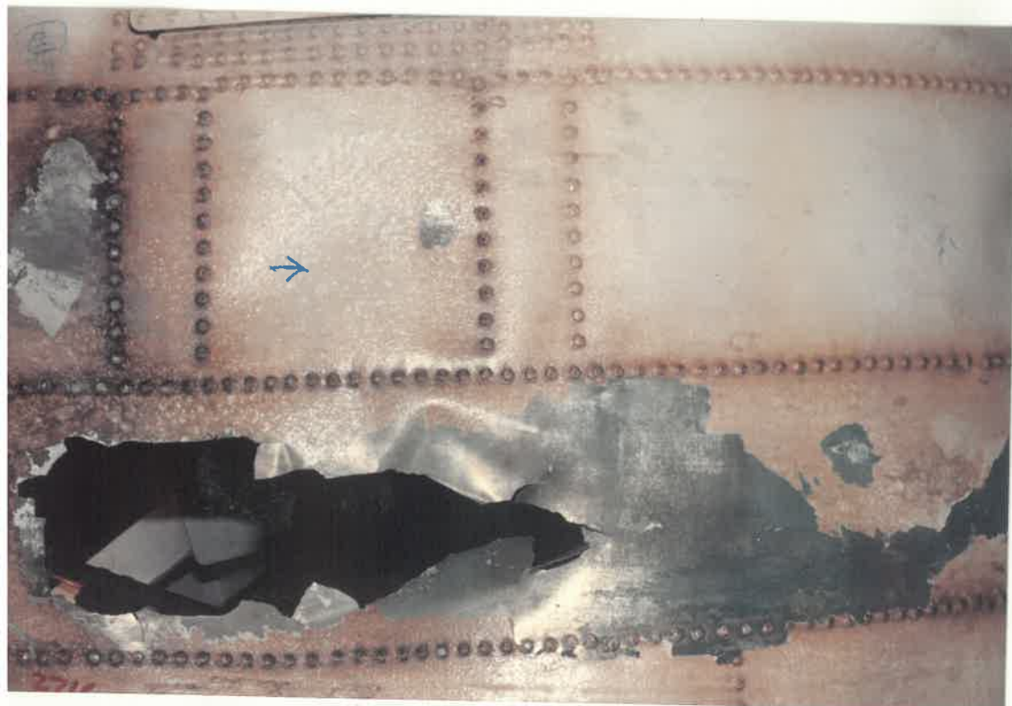
BURNT TAIL SECTION - ANOTHER EXTERNAL VIEW
