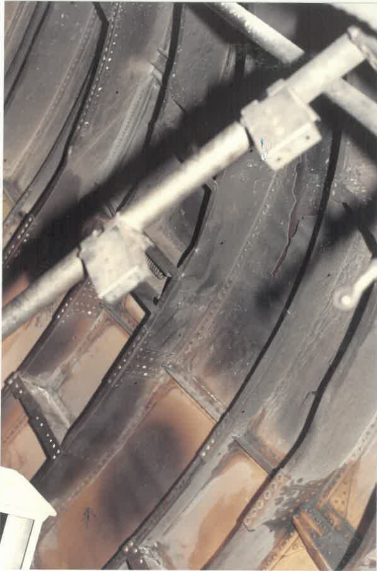
TAIL SECTION INTERNAL DAMAGE - ANOTHER VIEW
