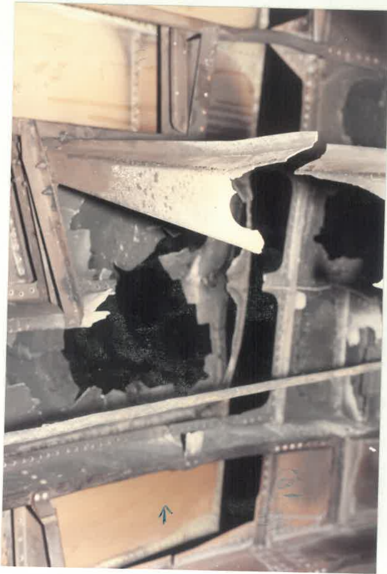
INTERNAL DAMAGE CAUSED DUE TO FIRE IN TAIL SECTION
