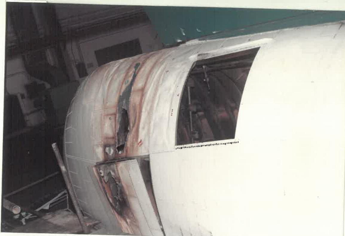
BURNT TAIL SECTION. BETWEEN 2 TO 3 O'CLOCK POSITION.
