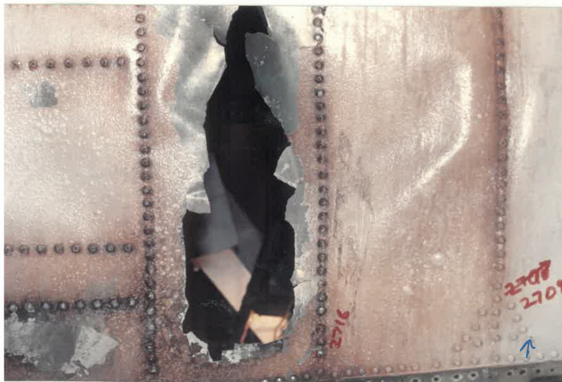
EVIDENCE OF BURNING BUCKLING AND DISCOLORATION DUE TO HI-TEMP.
