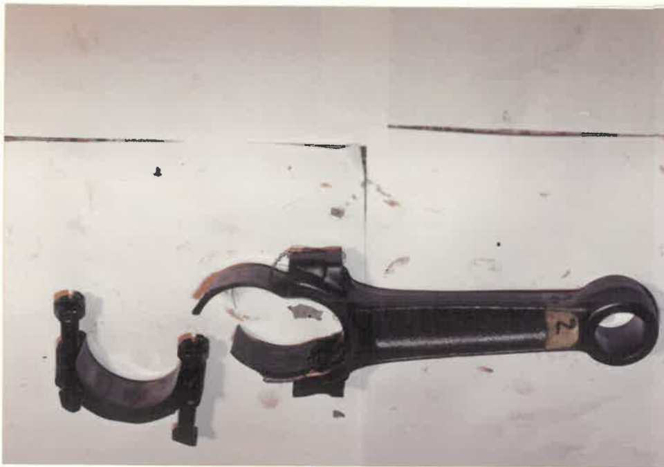
NO.2 CONNECTING ROD. NOTE:- WELDED BEARING.
