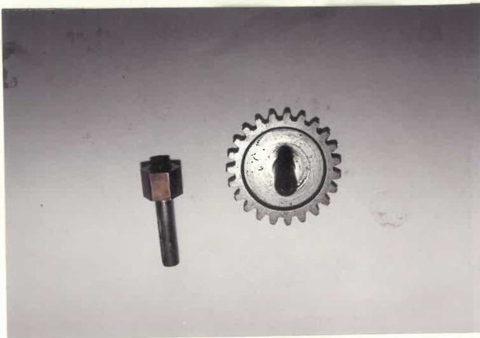
TACHOMETER GEN DRIVE. NOTE:- SHEARED SHAFT.
