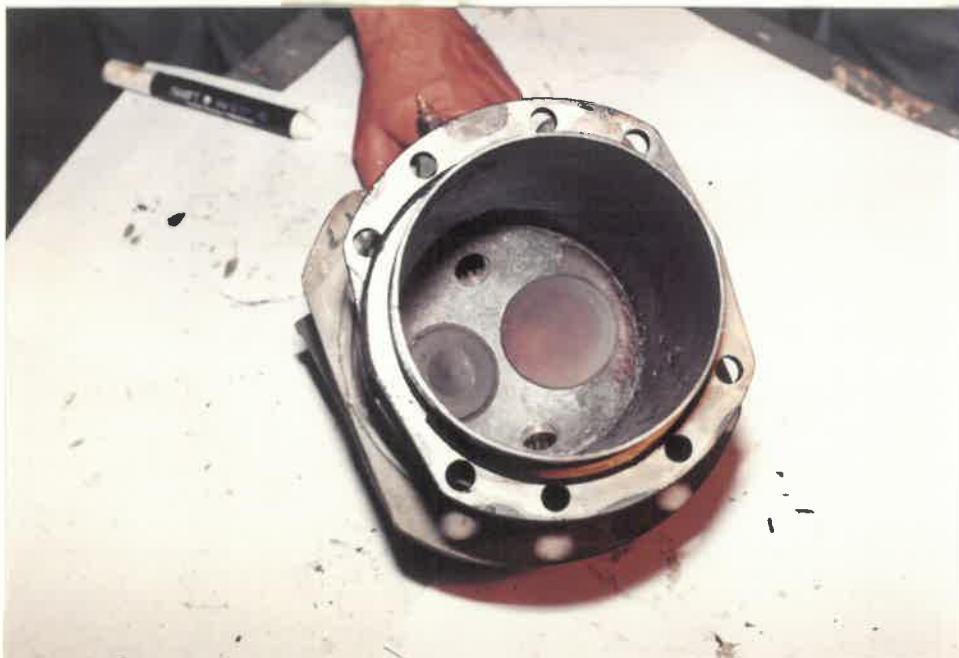
CYLINDER SLEEVE. NOTE:- INTERNAL SCORING.
