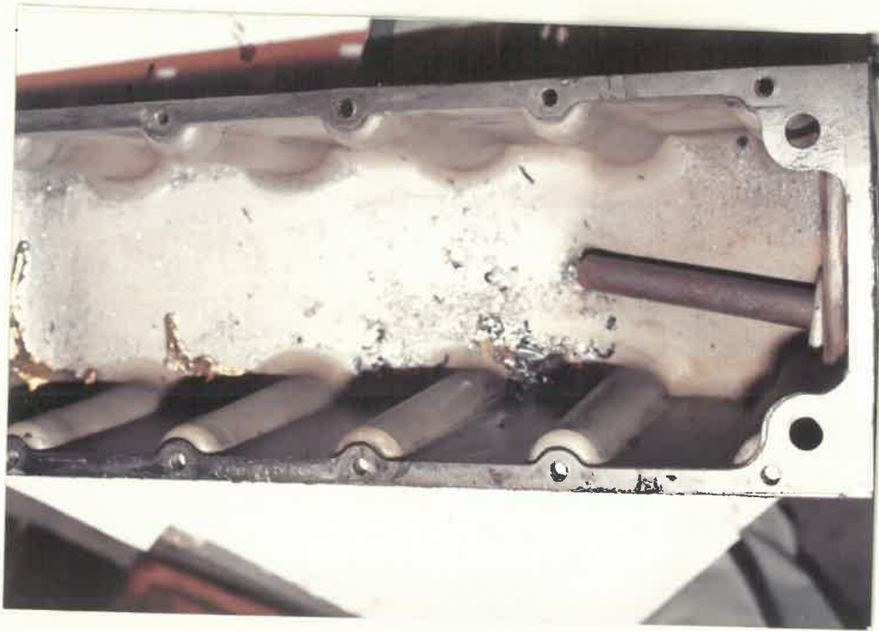
OIL SUMP. NOTE:- METAL DEPOSITS.
