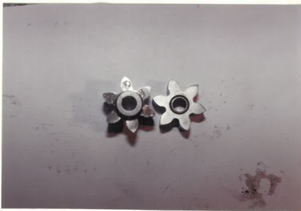
OIL PUMP GEARS. NOTE:- SCORING AND SCRATCH MARKS.
