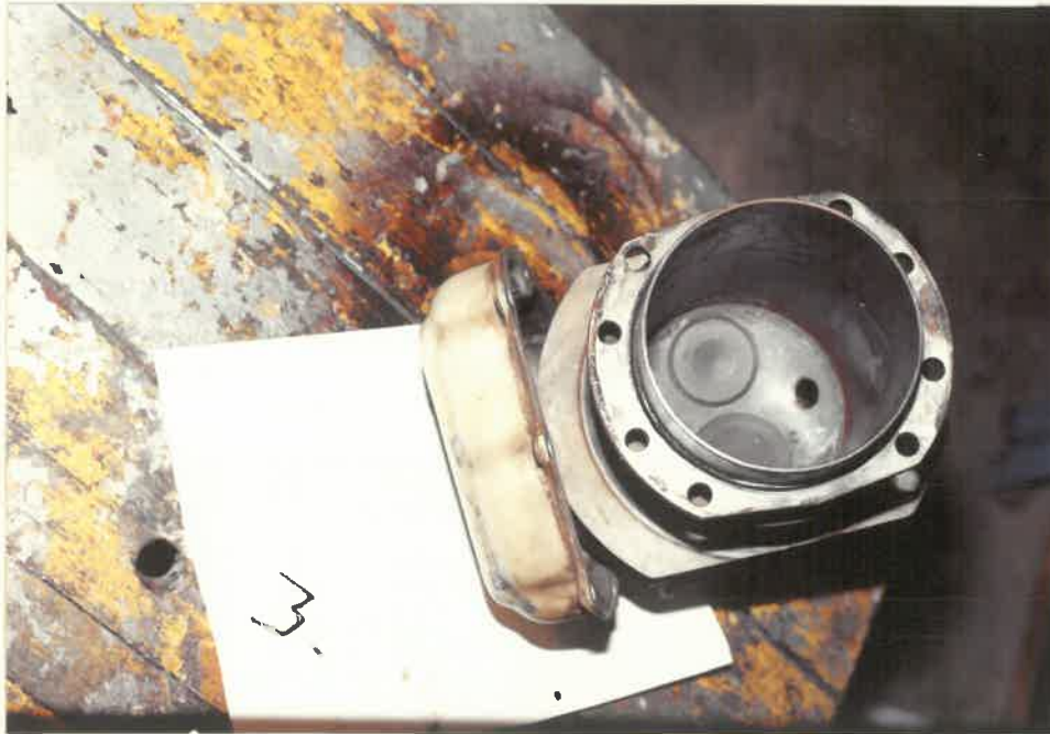
CYLINDER SLEEVE. NOTE: INNER WALL SCORING
