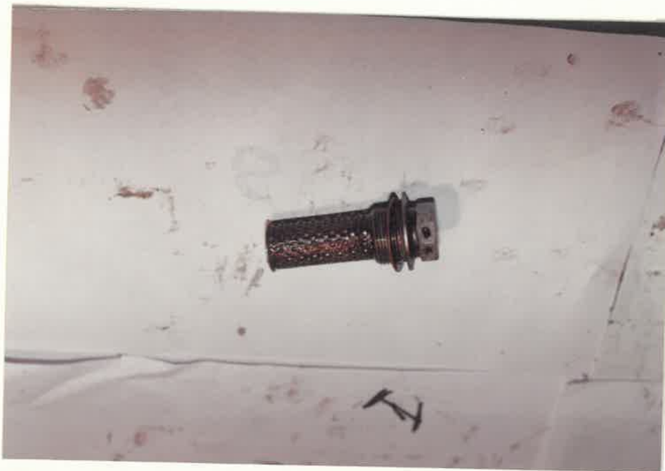
SCAVENGE OIL FILTER. NOTE:- DISINTEGRATED ELEMENT.
