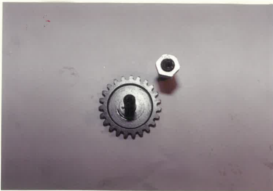
OIL PUMP GEARS. NOTE:- SCRATCH MARKS.
