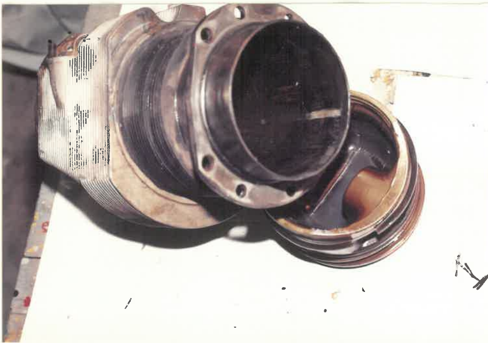
NO.1 CYLINDER. NOTE:- INTERNAL SCORING.
