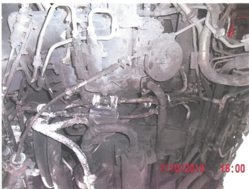
Detailed View of Damages on Lower Side of Engine
