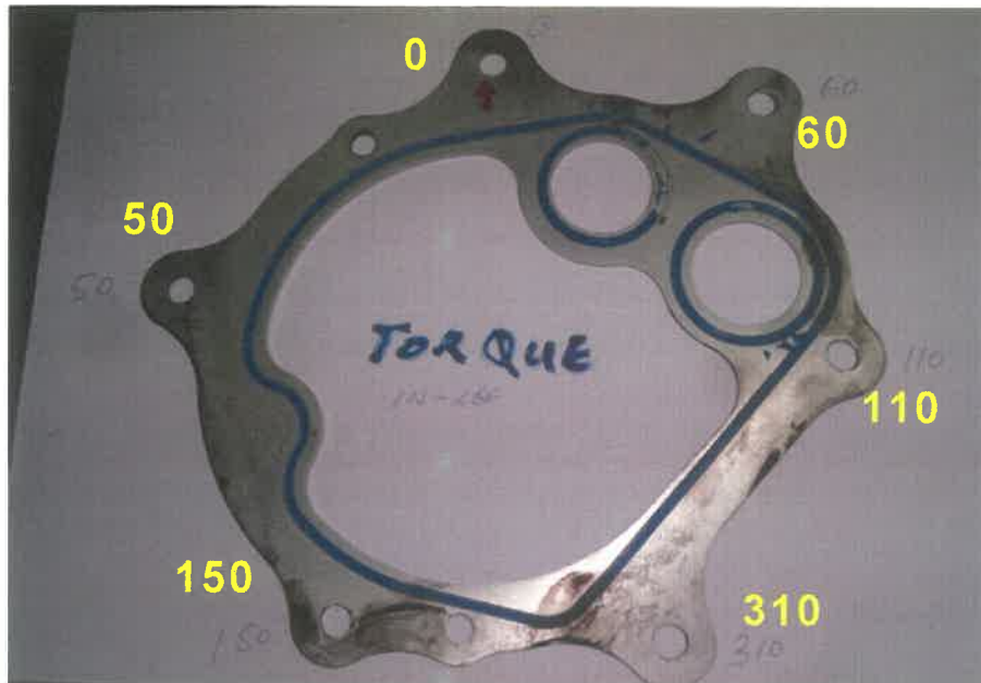
Measured Un-seated* Torque Values of MEC Mount Nuts
