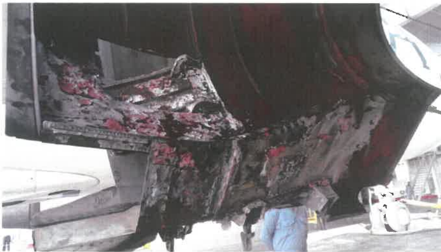
Left Hand Thrust Reverser Cowl Damage
