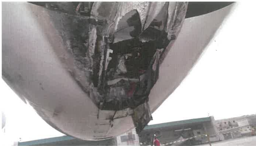
Thrust reverser cowlings lower side damage from in-flight fire
