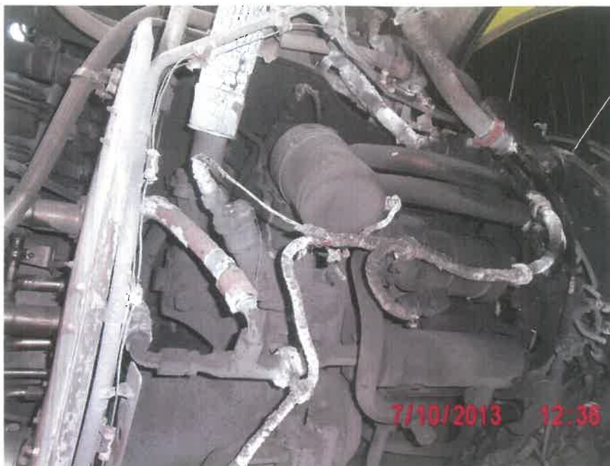
Wiring Damaged by In-Flight Fire on Lower Right Side of Engine
