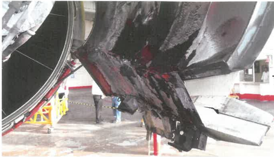
Right Hand Thrust Reverser Cowl Damage
