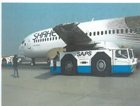
Stable movable wing support arrangement
