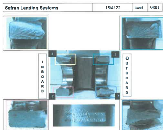
Figure 5: Overview of the retraction bracket (PN 201478286; SN HSM/DAM/0127/93) confirming the fracture of two lugs. The fracture surfaces were arbitrarily numbered from 1 to 4.
