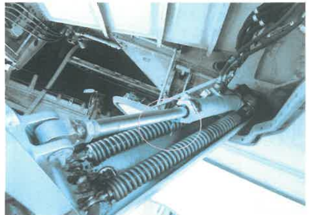
RMLG Lockstay Actuator, Protruded seal
