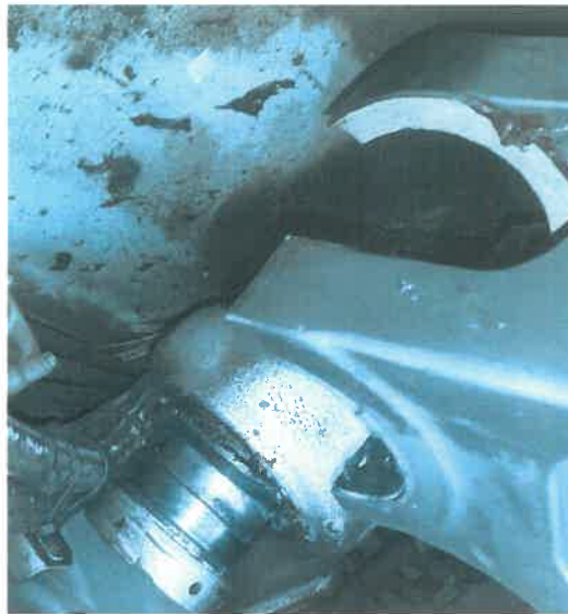
On aircraft close up view of the failed Retraction Bracket
