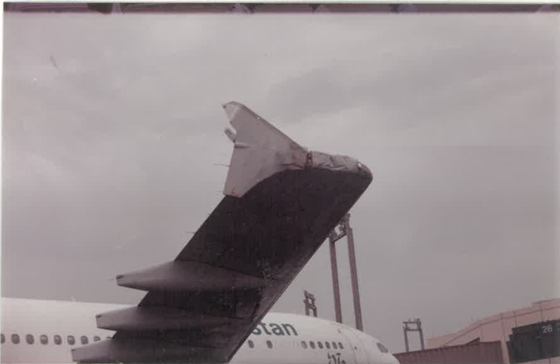
RT WING DAMAGE CAUSED DUE TO AVIOBRIDGE NO.25 STRIKING IN THE INCIDENT.
