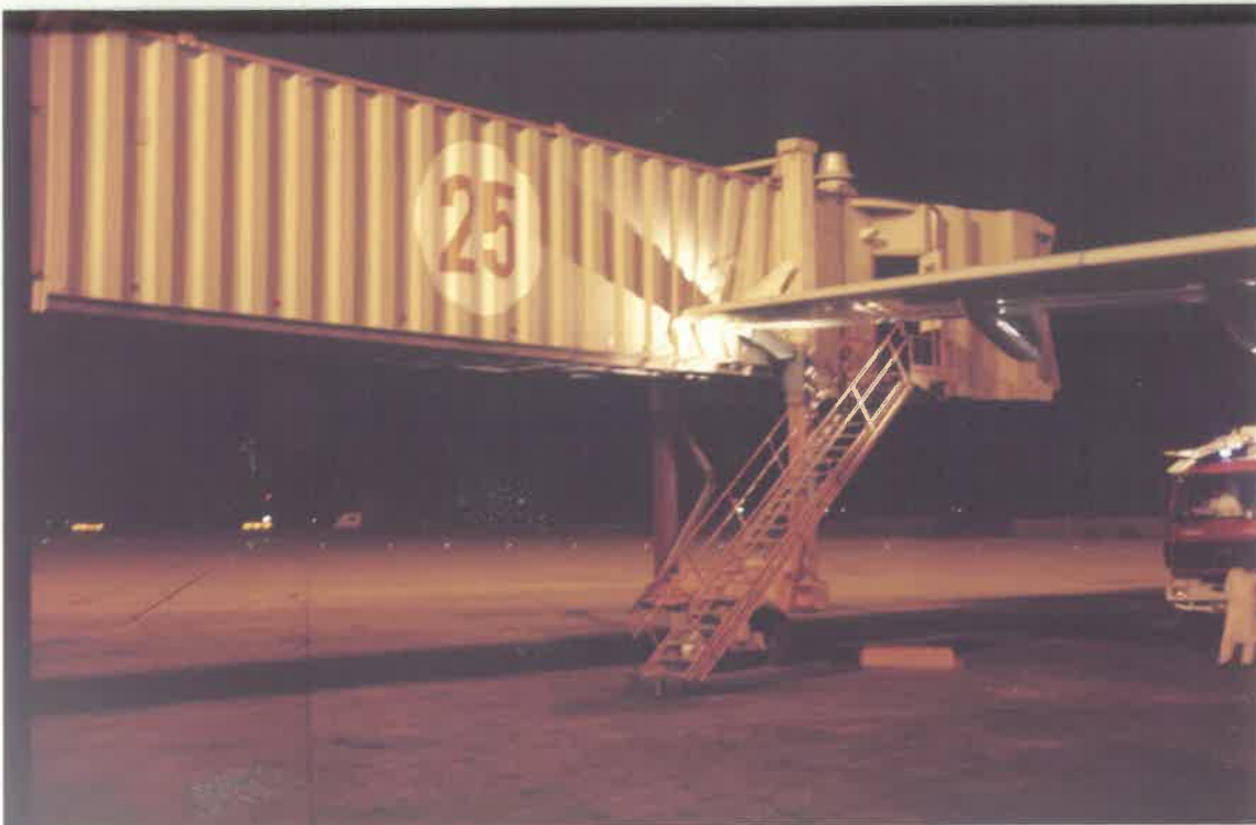
AVIOBRIDGE NO.25 AFTER IT COLLIDED WITH RT WING OF AIRBUS PARKED AT GATE NO.26.
