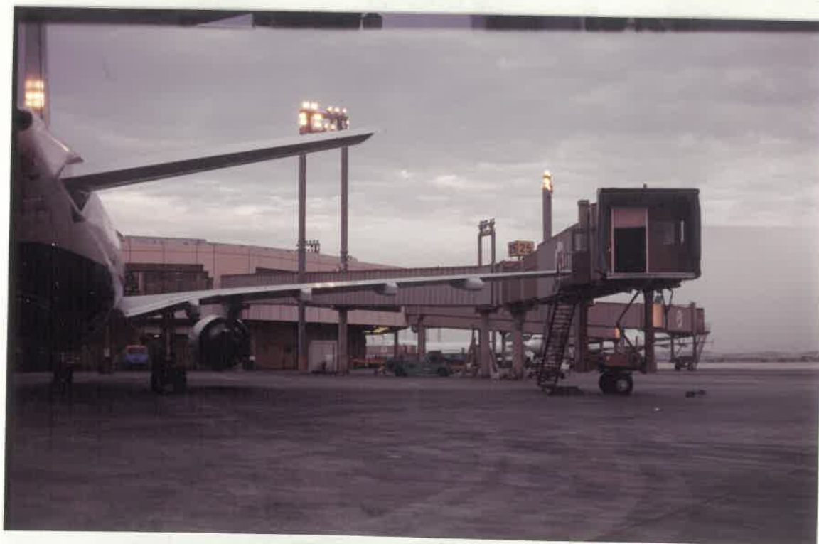
AVIOBRIDGE NO.25 COLLIDED WITH RT WING OF AIRBUS REG.NO.AP-BEC PARKED AT GATE NO.26 AFTER IT ROLLED ON ITS WHEEL DUE TO STRONG WIND. NOTE: SEE PLB WHEEL POSITION.
