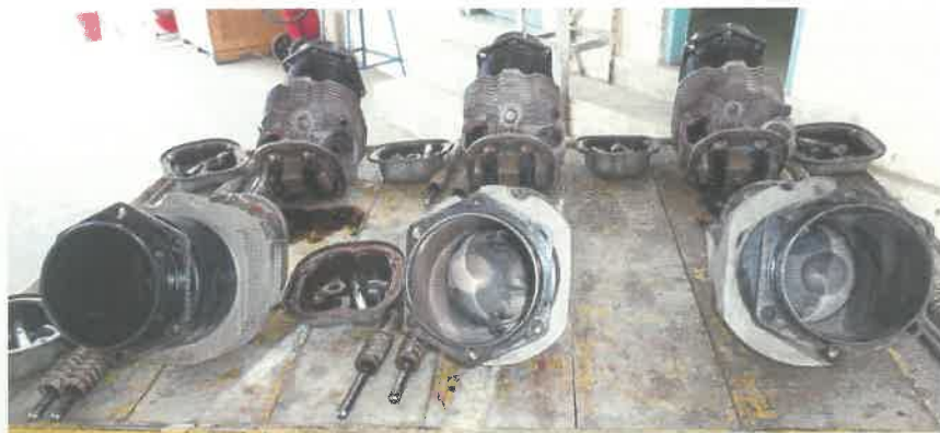
No scoring, scratches or overheating signs observed on inner side of 06 Cylinders along with their associated Parts
