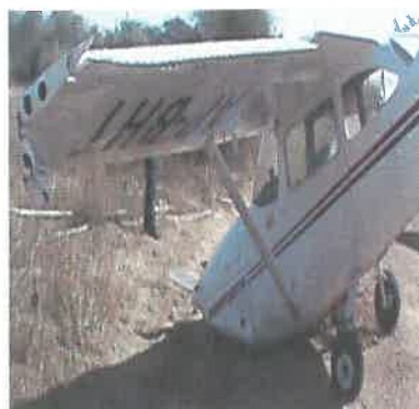
Fig 6: Minor Damage on Left Wing
