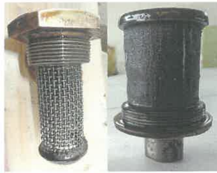
Undamaged and Unclogged Oil Filter
