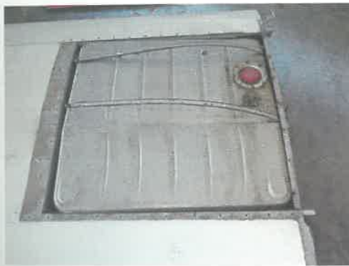
Properly Secured and un-damaged Left Wing Fuel Tank
