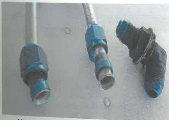
Undamaged fuel pipes and elbow union fairings
