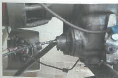
Undamaged Oil Filter Housing
