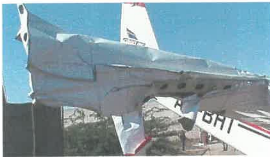
Fig 2: Right Wing Structure severely damaged
