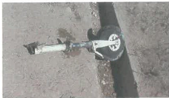
Fig 3: Nose Landing Gear broke in air after hitting the concrete wall
