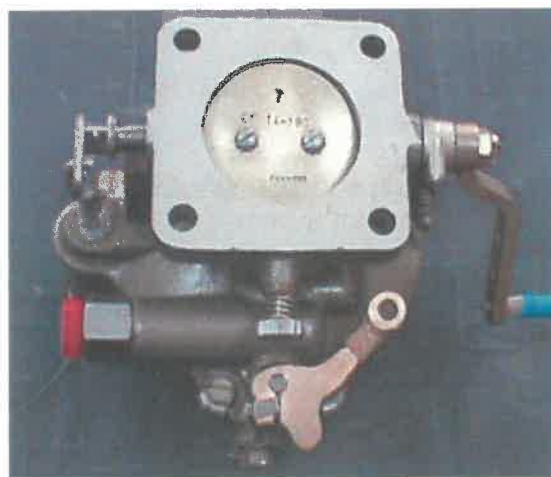
A serviceable carburettor, showing state of throttle lever and piston when the butterfly valve is at fully closed position
