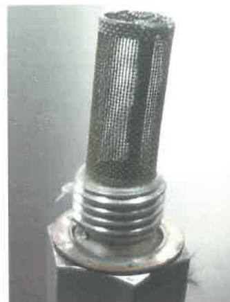
Carburettor Inlet Filter Undamaged and Unclogged
