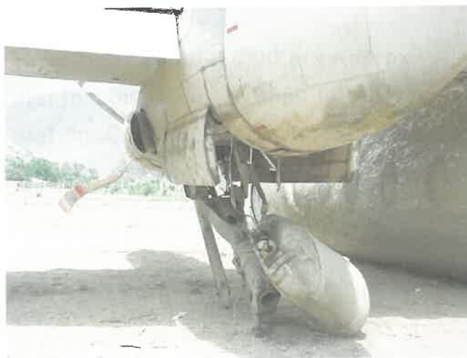
HULL FRACTURES ON FLOOR
