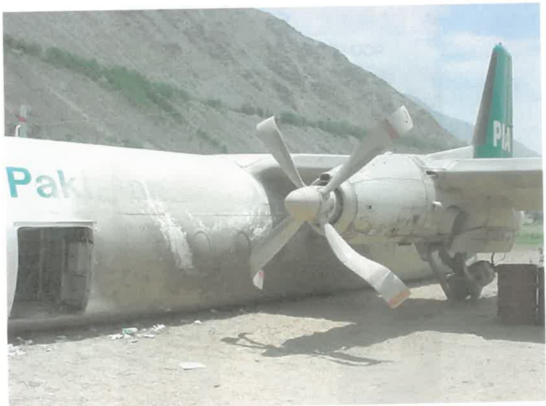
LANDING GEARS BROKEN & ENGINE PROPELLER DAMAGE
