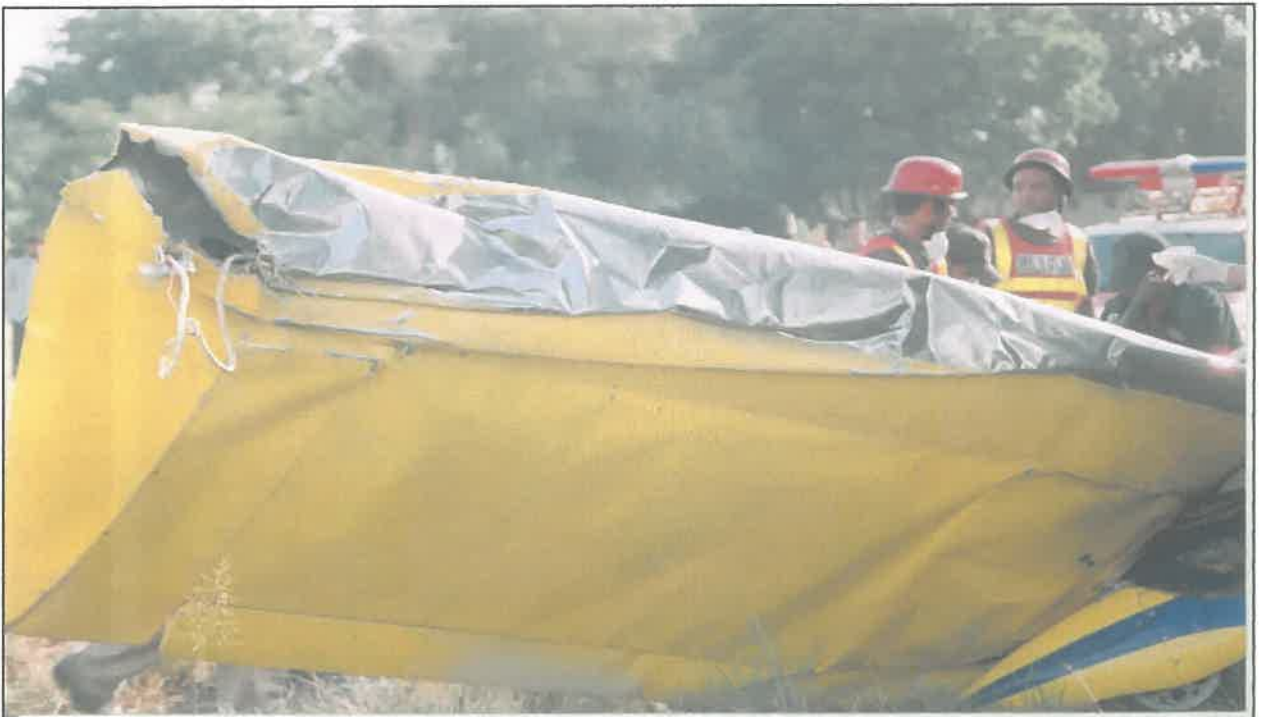
RIGHT WING LEADING EDGE PAINT FLAKED OFF BUT NO TELESOPING
