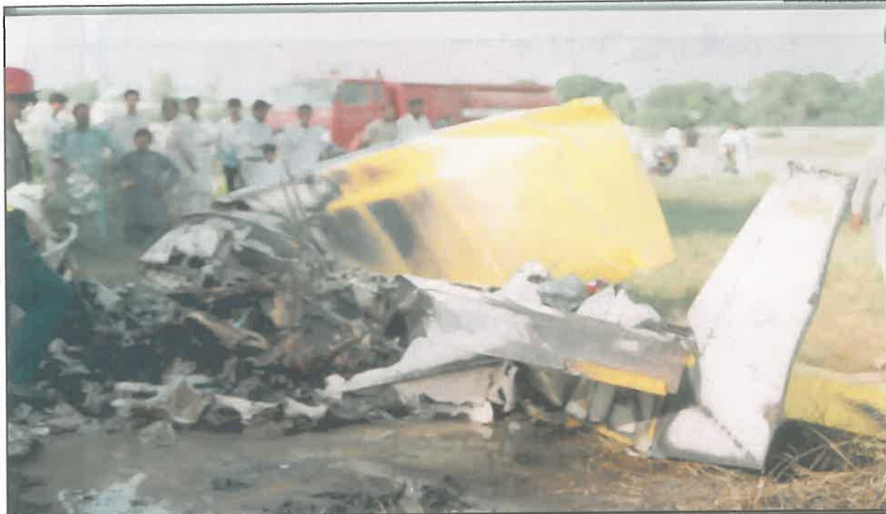
MAIN WRECKAGE EXTENSIVE BURNING IN CENTRE TAIL AND RT WING UN- BURNT
