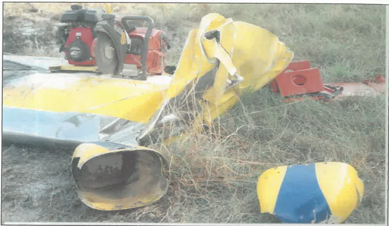
LEFT WING TIP BENT ON INITIAL IMPACT AND NOSE TIP SEPARATED
