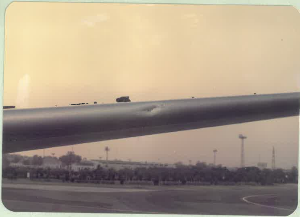
VIEW OF DENT ON LEADING EDGE OF LEFT HORIZONTAL STABILIZER.
