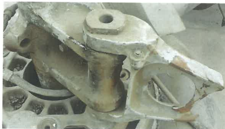
Fractured Lower Torsion Link
