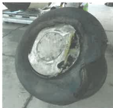
Rubbing marks on wheel hubs
