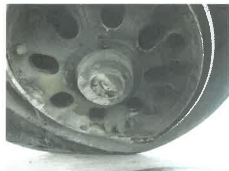
Rubbing marks on wheel hubs
