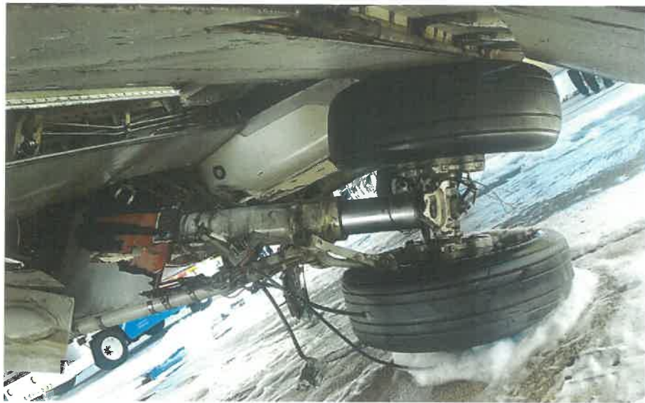
Close up of the collapsed left main landing gear
