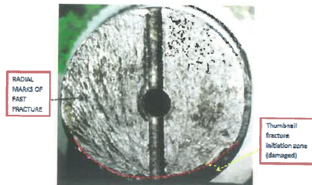
Close up view of fracture surface
