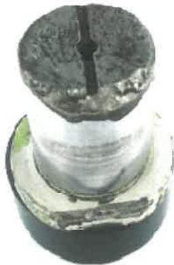
Fractured Connecting Pin
