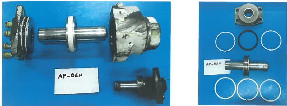
Shimmy damper internal seals and mechanism were found intact
