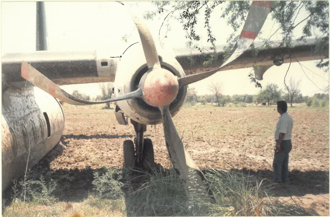
PORT ENGINE PROPELLER TIPS SHOWING FORWARD BENDING
