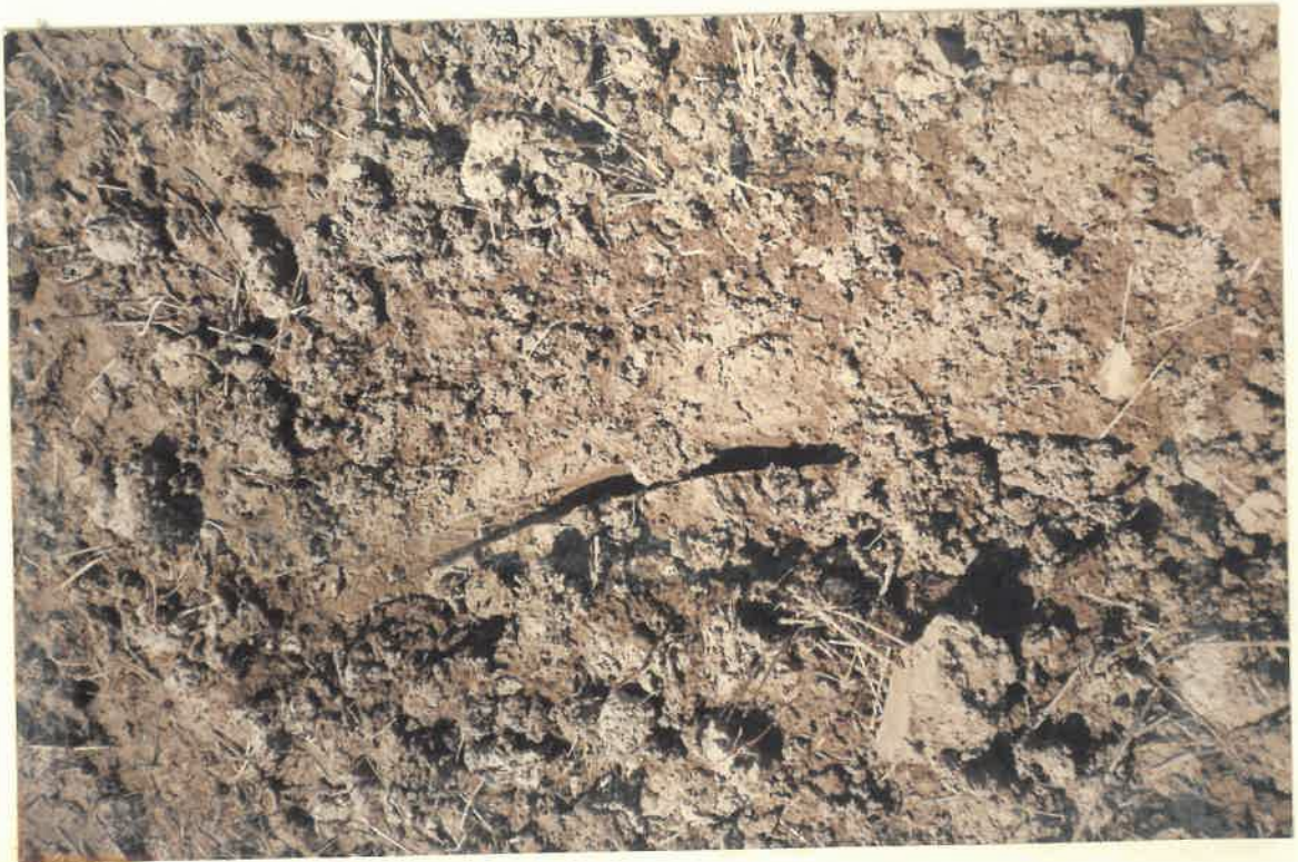
SLASH MARK MADE BY PORT PROP AT INITIAL IMPACT OF AIRCRAFT
