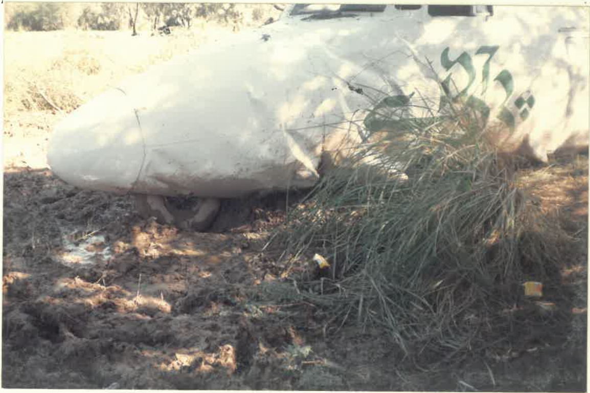
NOSE WHEEL NOT FULLY RETRACTED
