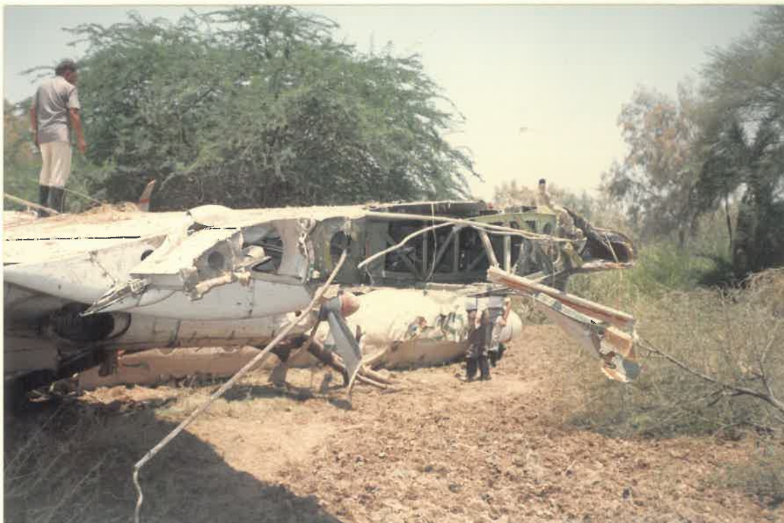
RIGHT WING BROKEN FROM MID SECTION
