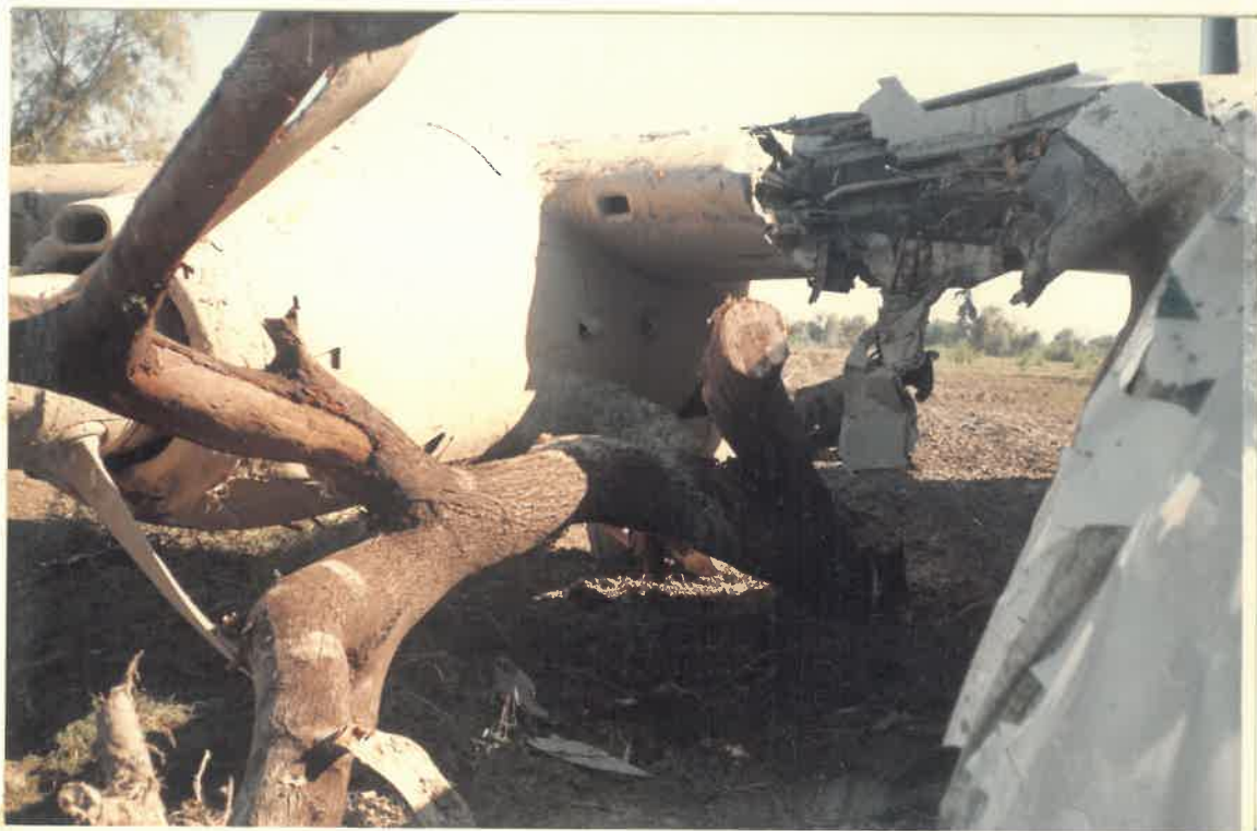
STARBOARD WING ROOT L.E. DAMAGED BY TREE
