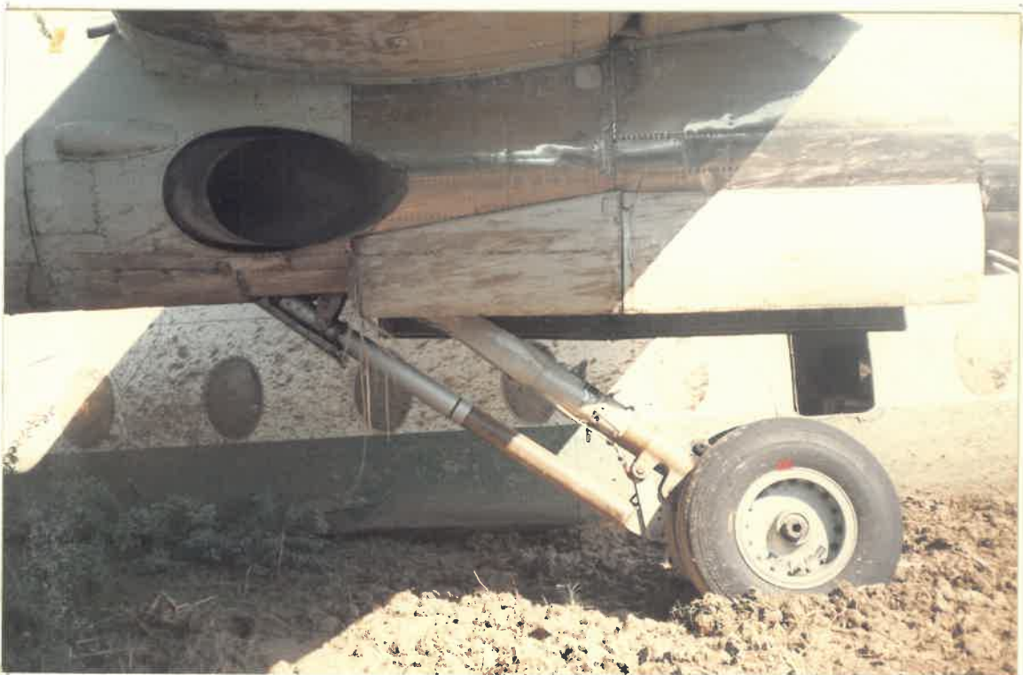
TREE BRANCHES STUCK IN LEFT MAIN GEAR DOOR
