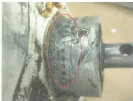
Ball bearing marks on actuator support surface.
