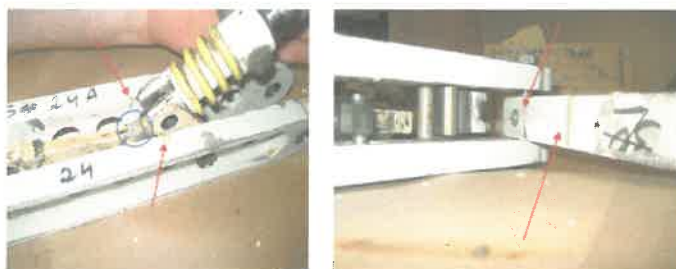
Marks on Brace from link bolt, link curl Marks on lower brace from hook/hook bolt
