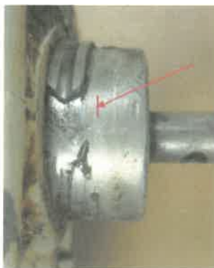
Marks showing inner bearing movement.
